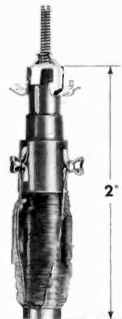
Fig. 18·15 Width coil. Inductance is 3 to 16 mh.
