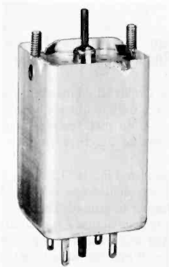
Fig. 16·11 Synchro-Guide transformer in shield can 1½ in. square. Top slug is blocking oscillator frequency adjustment for plate winding AC; bottom is waveform adjustment for stabilizing coil CD. (Merit Coil and Transformer Corp.)
