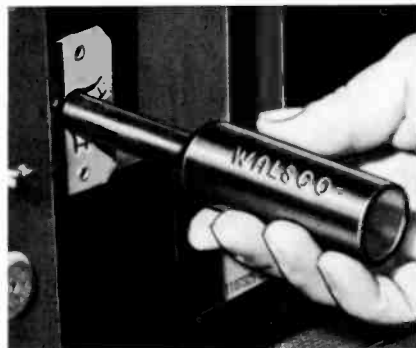
Fig. 25·25 High-voltage cheater being inserted at back of color television receiver. (Walsco Electronics Co.)
