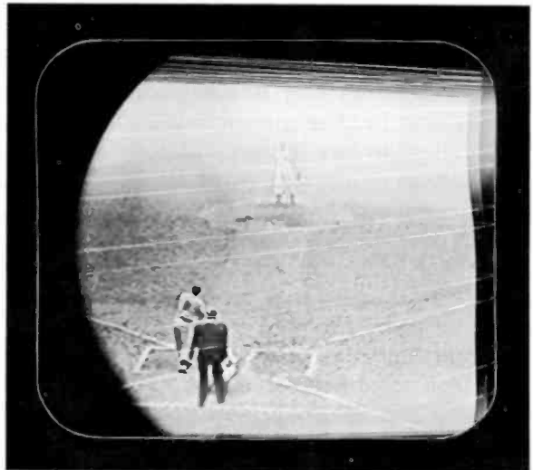
Fig. 14·21 Bend only at top of picture, with straight edge at side of raster. (RCA.)
