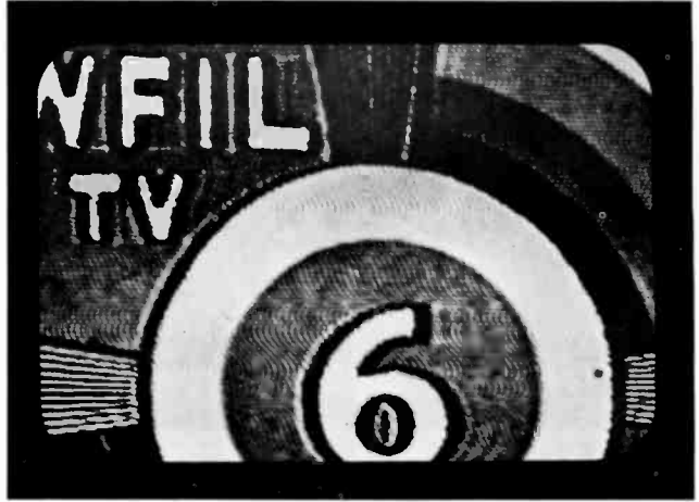
Fig. 23·5 Fine herringbone-weave or wormy effect of 4.5-Mc beat in picture. (RCA.)
