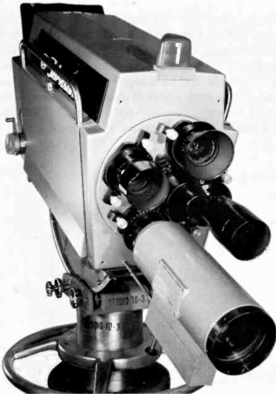
Fig. 2·2 Television camera with four lenses of different focal lengths mounted on a revolving turret. The long barrel has a zoomar lens for extreme close-ups. An image orthicon camera tube is used in this camera head. (RCA.)
