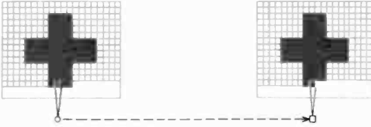
Fig. 1·2 Reproducing a picture by duplicating its picture elements.
