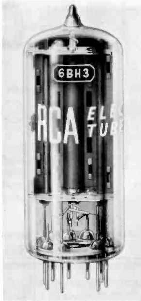
Fig. 6-12 Half-wave power rectifier tube 6BH3 for damper diode in horizontal output circuit. This is a novar tube with dark heater. (RCA.)
