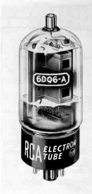
Fig. 6-11 Horizontal power output tube with octal base. Top cap is the plate. (RCA.)
