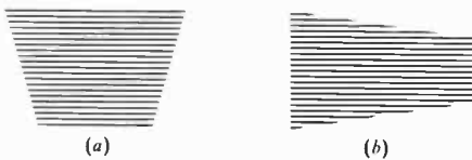
Fig. 3·6 Trapezoidal raster. (a) Keystoned sides caused by unsymmetrical horizontal scanning. (b) Keystoned at top and bottom because of unsymmetrical vertical scanning.
