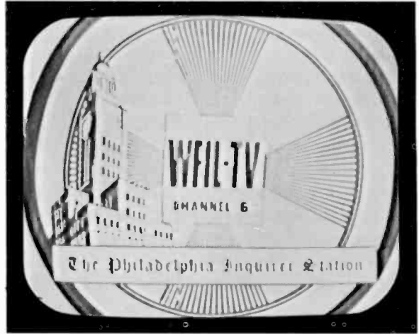
Fig. 9·13 Test pattern illustrating loss of low-video signal frequencies. Background is weak, lettering is not solid, and the side wedges have weaker intensity than the wedges at top and bottom. (RCA Pict-O-Guide.)
