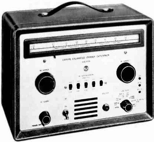
Fig. 20·15 Crystal-calibrated marker, oscillator. (RCA.)
