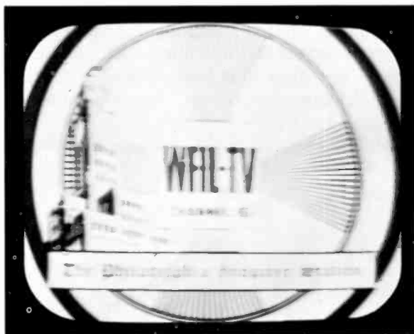
Fig. 9·12 Test pattern illustrating loss of high video frequencies. Note the lack of separation of the divisions in top and bottom wedges. Also they have weaker intensity than the side wedges. (RCA Pict-O-Guide.)
