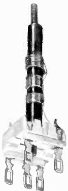
Fig. 22·16 Construction of ratio detector transformer. (Meissner Mfg. Division.)
