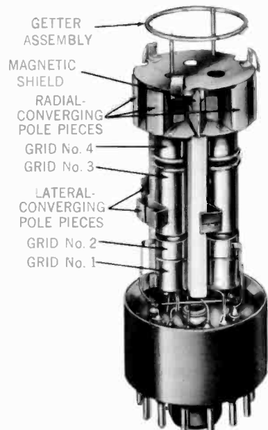
Fig. 25·18 Assembly of three electron guns in 21FJP22 color kinescope. (RCA.)
