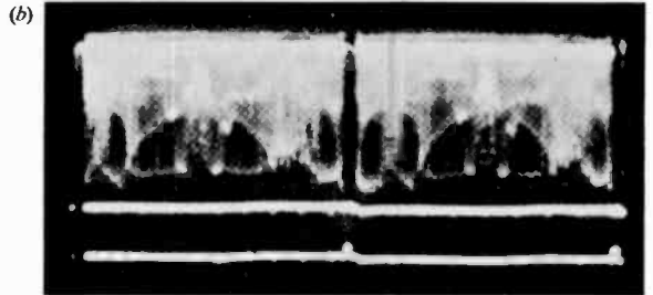
Fig. 4·7 Typical oscilloscope photographs of composite video signal shown with sync polarity downward. (a) Two lines of horizontal picture information between horizontal blanking and sync pulses. Oscilloscope sweep at 7,875 cps. (b) Two fields of vertical picture information between vertical blanking and sync pulses. Oscilloscope sweep at 30 cps.
