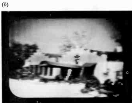
Fig. 4·9 Effect of video frequencies on picture reproduction. (a) Normal picture reproduction. (b) Only large areas in picture reproduced by low video frequencies up to 0.1 Mc. (c) Only horizontal edges and outlines reproduced by high video frequencies between 0.1 and 4 Mc.
