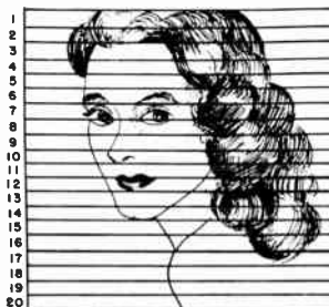
Figure 9. How linear scanning is accomplished.
