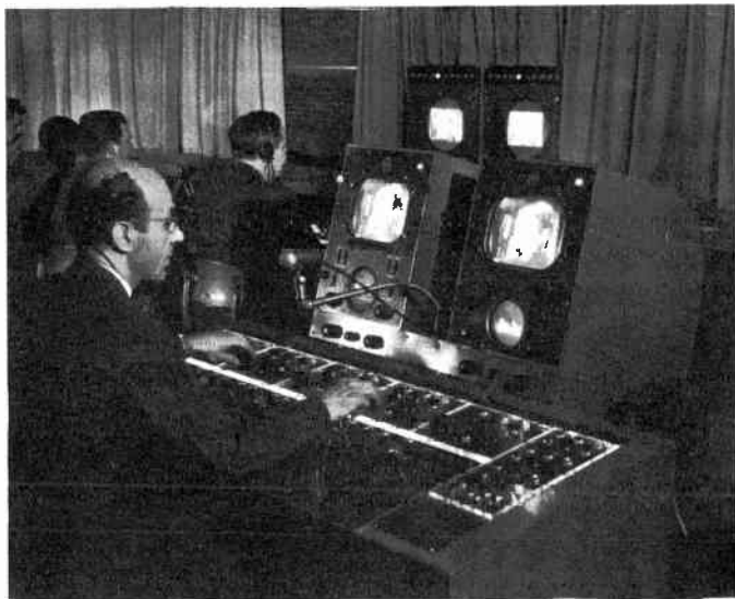
Figure 21. The technical director operates the switching panel and selects the desired camera. (courtesy NBC)
