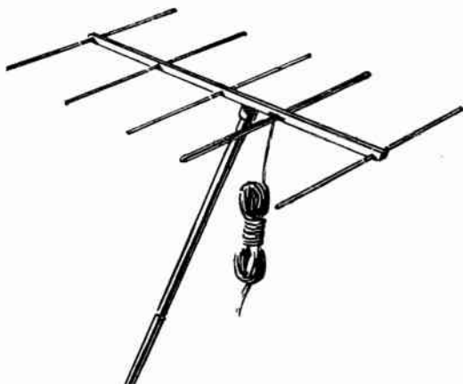
Figure 35. High-gain, five-element array, suitable for reception of single high band television station. (courtesy Roger Television)
