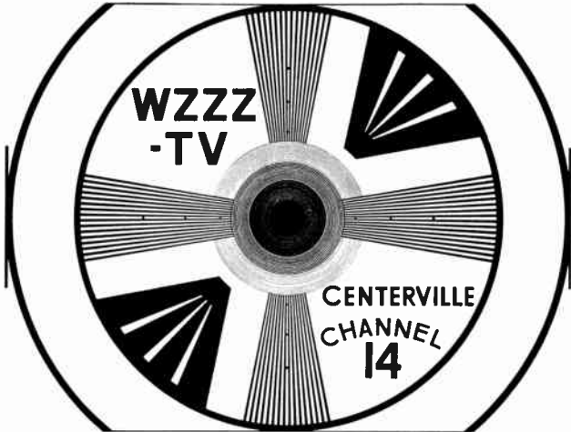
Figure 12. Pattern obtained from monoscope tube.
