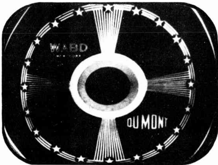
Figure 54. Test pattern showing negative picture caused by improper polarity of grid of picture tube.
