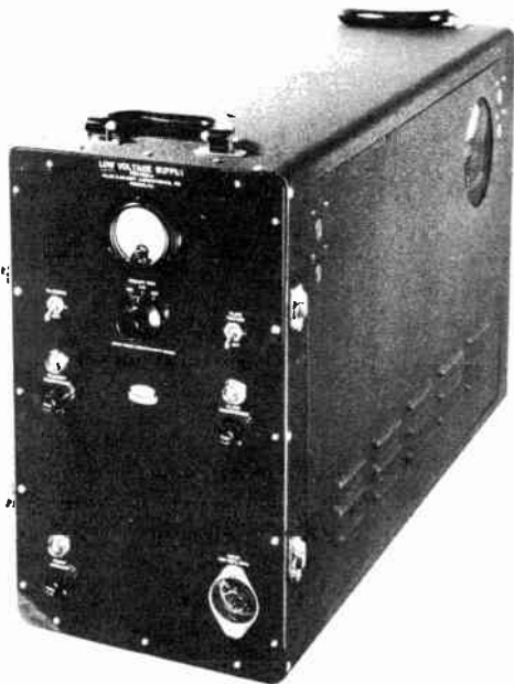
Figure 74. Low-voltage supply. (courtesy DuMont)
