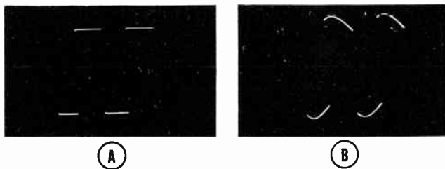
Figure 69. Square wave patterns obtained when checking low-frequency response of video amplifier. A. Good low-frequency response, B. Poor low-frequency response.
