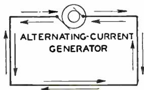
ALTERNATING CURRENT FLOWING IN CLOSED CIRCUIT
