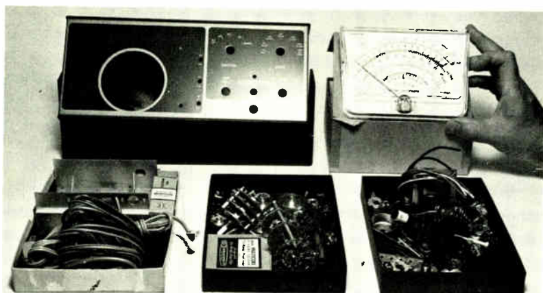
5-6. Major components of typical VTVM kit. Back: panel, chassis, and meter. Front: wire, switches, resistors, capacitors, etc., in old film boxes.
