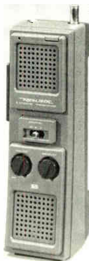
18-6. People who are accustomed to using the telephone like this type of mobile CB transceiver because the handset fits naturally in their palms. A built-in loudspeaker can be switched on to let other passengers in the car hear conversations. The Radio Shack CB-Fone, Model TRC-56.
