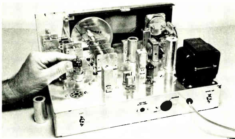
8-6. Top view of completed HR-10B chassis. Layout is clean and open. Heavy power transformer is at right. Empty socket at left is for a 100-kc crystal calibrator, an optional accessory.
