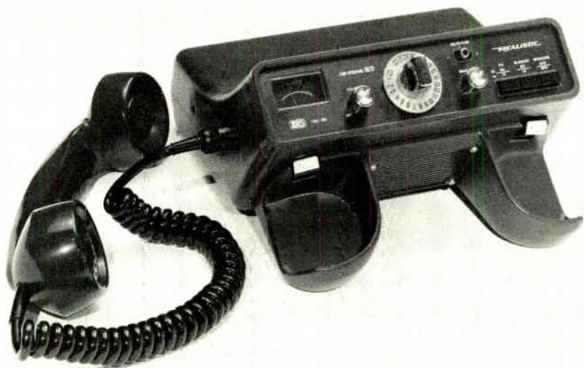
18-6. People who are accustomed to using the telephone like this type of mobile CB transceiver because the handset fits naturally in their palms. A built-in loudspeaker can be switched on to let other passengers in the car hear conversations. The Radio Shack CB-Fone, Model TRC-56.
