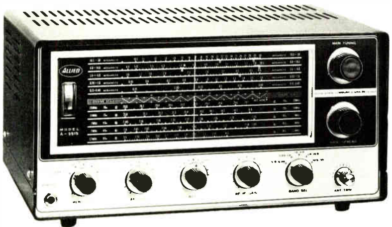
8-13. This five-band solid-state receiver, the Allied Model A-2515, provides general shortwave coverage as well as bandspread on the popular amateur bands.
