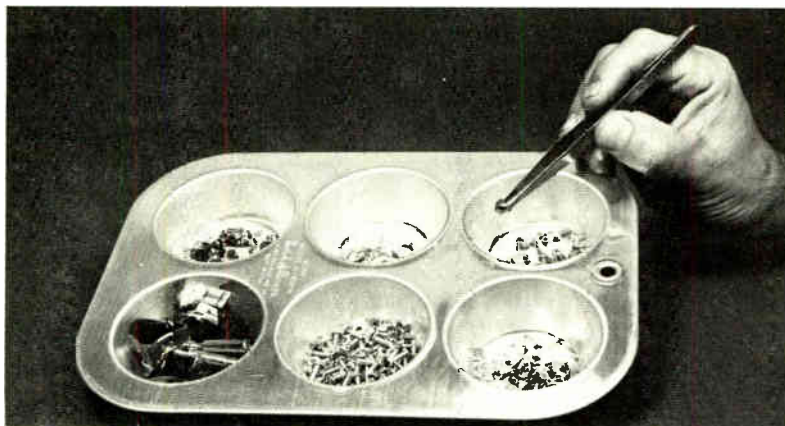
5-7. A muffin tin is an excellent holder for nuts and bolts and other small hardware of kit or other construction projects. Note use of tweezers for picking up tiny parts.
