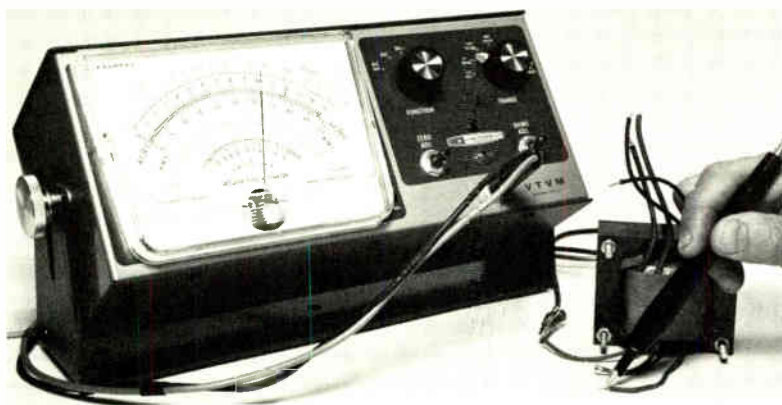
5-24. A completed VTVM in a typical application: checking the continuity of a power-transformer winding. The meter reads 180 ohms; top resistance scale, multiplied by ten in accordance with setting of range switch in the upper right-hand corner of the panel.
