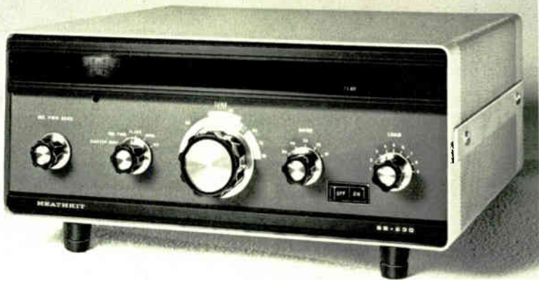
11-11. Called a "linear," the SB-230 boosts SB-104 power to 1000 watts.
