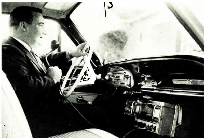
13-5. A telephone operator's chest-type microphone lends itself to mobile use because it remains in correct speaking distance from the driver's mouth. He presses switch on the mike's base to actuate the transmitter, under the dash. Receiver is farther to left.
