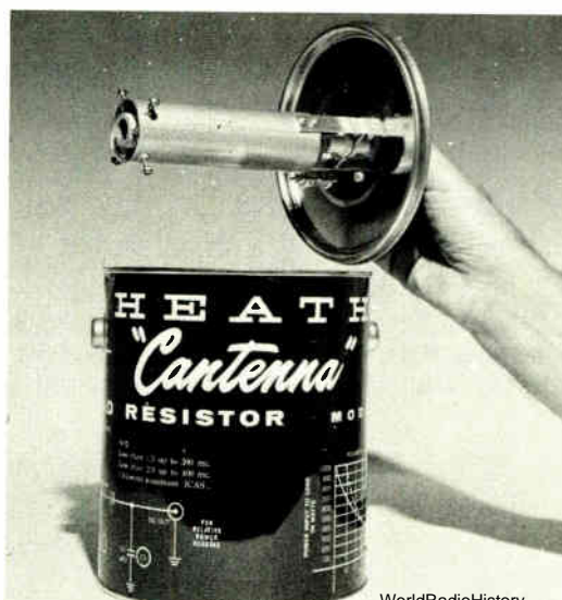
12-6. The heart of this dummy antenna is a large resistor, inside a protective aluminum tube fastened to the lid of the gallon can. The latter is filled with mineral or transformer oil to dissipate heat in the resistor created by energy from the transmitter to which this useful item is wired.
