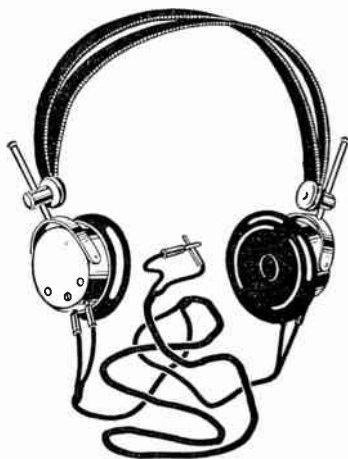
FIG. 18.—A pair of phones, showing head-band, leads and tips.
