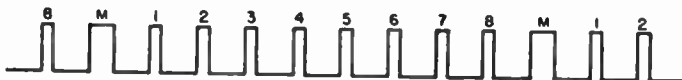
Fig. 8—Time-multiplex train of subcarrier pulses for 8 channels and marker pulse M for synchronization of receiver with transmitter.
