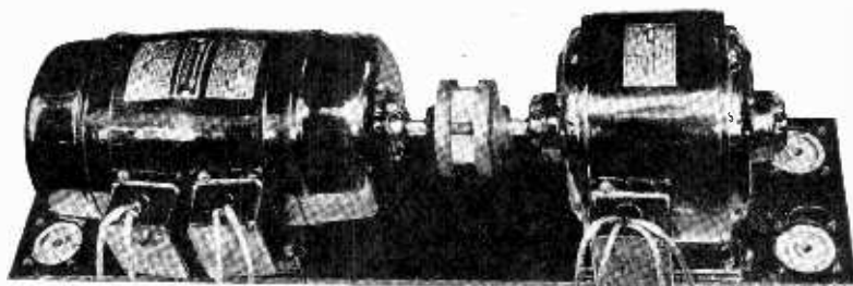
FIG. 337. Motor Generator Set for Model ET-8003 Transmitter.
