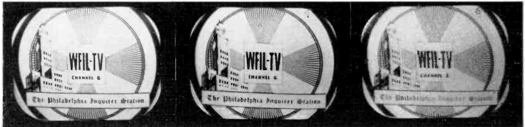
Fig. 23. Typical picture shown for (a) strong, (b) medium, and (c) weak signal strength;
