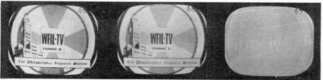
Fig. 28. Interference due to local oscillator radiation from another TV receiver viewed under conditions of (a) strong, (b) medium, and (c) weak reception.
