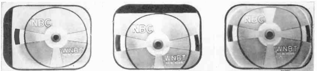
Fig. 13 (left). Horizontal centering control misadjusted. Fig. 14 (center). Vertical centering control misadjusted. Fig. 15 (right). Vertical linearity control misadjusted.
