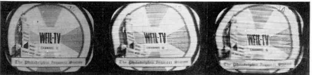
Fig. 24. Adjacent channel interference under conditions of (a) strong, (b) medium, and (c) weak reception.
