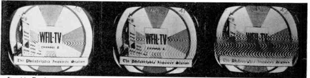
Fig. 30. Diathermy interference viewed under conditions of (a) strong, (b) medium, and (c) weak reception.
