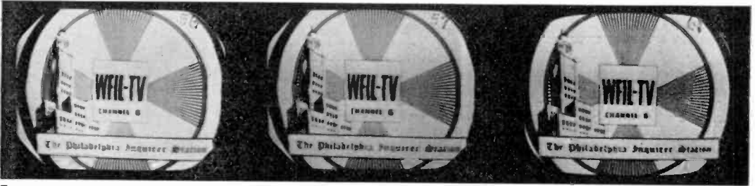
Fig. 29. Electric razor interference viewed under conditions of (a) strong, (b) medium, and (c) weak signal reception.
