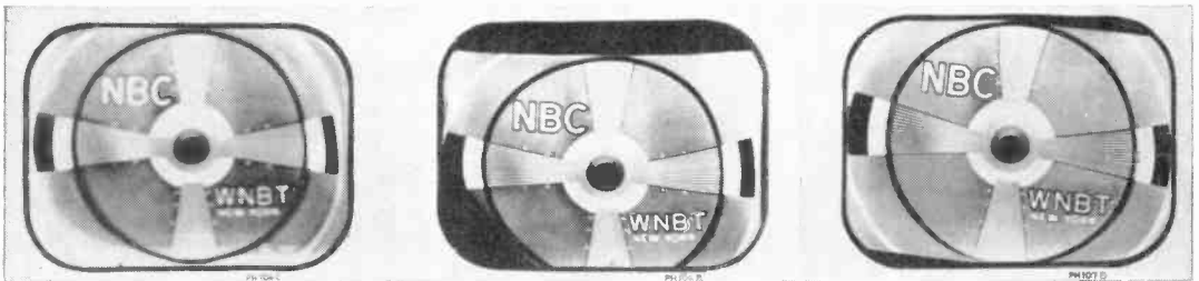
Fig. 10 (left). Focus control misadjusted. Fig. 11 (center). Focus coil and ion trap magnet misadjusted. Fig. 12 (right). Deflection yoke misadjusted (rotated).
