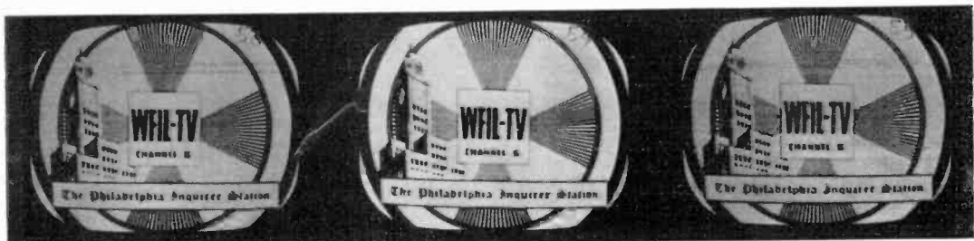
Fig. 27. Ignition interference viewed under conditions of (a) strong, (b) medium, and (c) weak reception.
