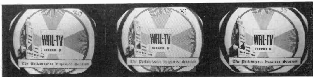
Fig. 26. FM image interference under conditions of (a) strong and (b) medium reception, and (c) with a series trap added.
