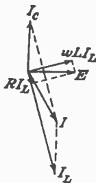
FIG. 44.—Vector diagram of current and voltage for capacity in parallel with resistance and inductance.
