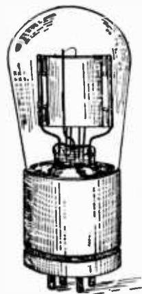
FIG. 8.—Vacuum tube showing contact prongs.
