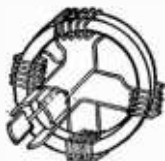
FIG. 19.—Armature with four loops and attached commutator.
