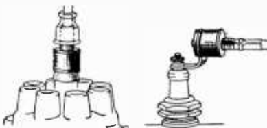
FIG. 16.—Resistances to eliminate interference.
