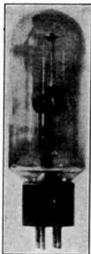
FIG. 7.—Photo-glow tube and its characteristic curves.
