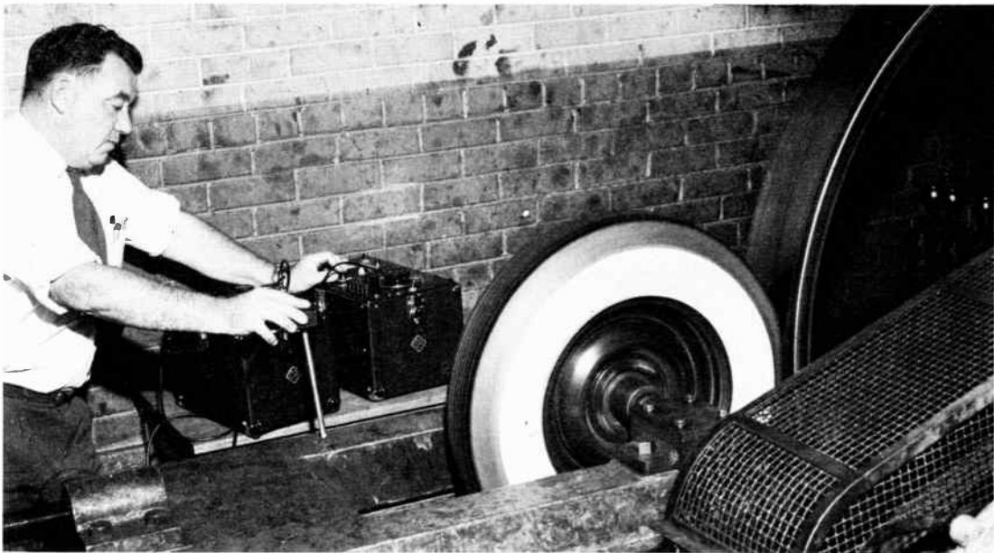
Figure 12-1. The vibration meter and analyzer are used here to determine the amount of vibration absorbed by a new Gates tire. The tire is taking extreme punishment from a cleat on the large wheel, which is traveling so fast that the cleat cannot be seen.
