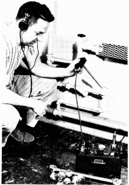
Figure 12-6. Checking a steam trap with vibration-measuring equipment.
