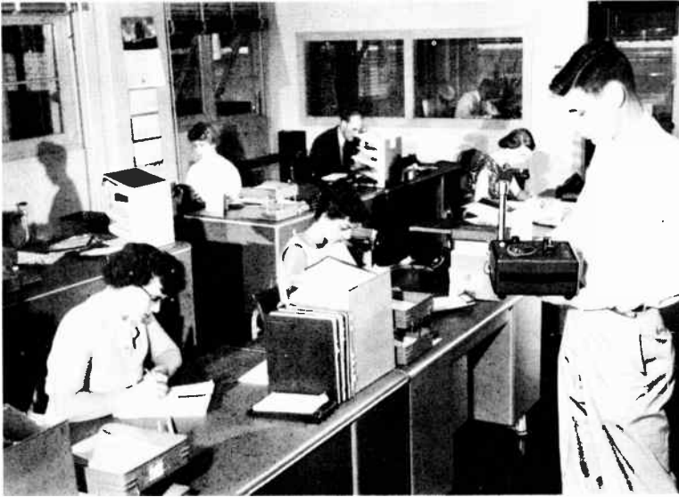
Figure 5-6. Another example of the sound-level meter in use: measuring over-all noise level in a commercial office.
