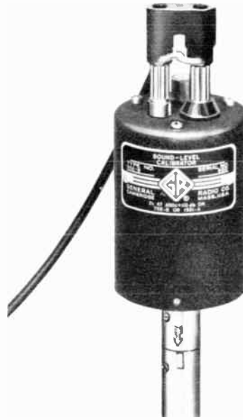
Figure 4-8. The Type 1552-B Sound-Level Calibrator placed on the microphone of a sound-level meter for calibration.
