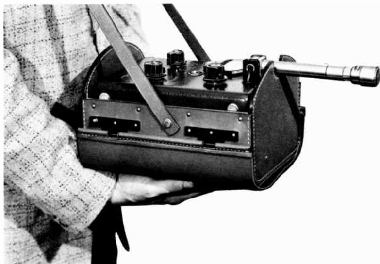
Figure 5-4. Hand-held operation of the sound-level meter.
