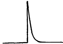
FIG. 10-11.—Form of the pulse produced by an abrupt change of direct voltage impressed upon the circuit of Fig. 10-10.
