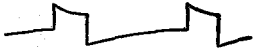
FIG. 10-26.—Typical wave form of condenser current or screen or suppressor voltage in the circuit of Fig. 10-25.
