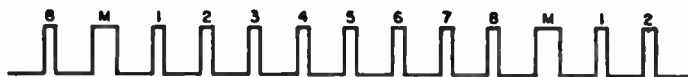
Fig. 10—Time-multiplex train of subcarrier pulses for 8 channels and marker pulse M for synchronization of receiver with transmitter.
