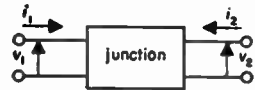
Fig. 13— Sign convention for defining the impedance and admittance of a 2-port junction.
