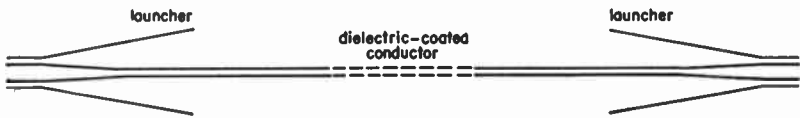
Fig. 17—Surface-wave transmission line with launchers at each end. These form transitions to coaxial line. Courtesy of Electronics
