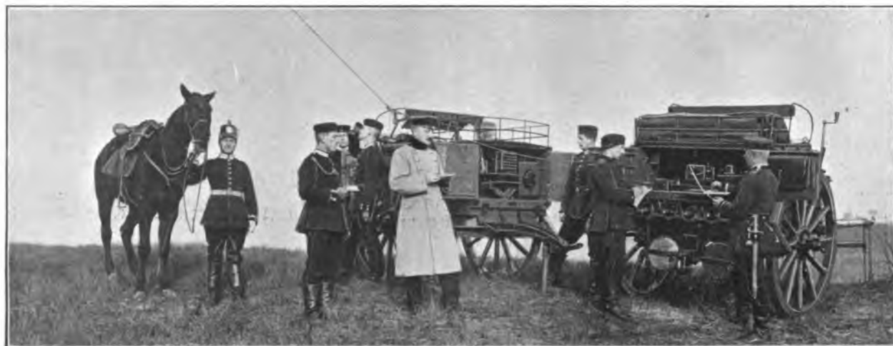
FIG. 76.—Portable Wireless Telegraphy Station—Train Unlimbered.
