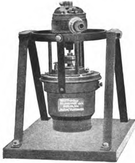
FIG. 37.—Mercurial Turbine Interruptor, with Cardanic Suspension, for Naval Stations.
