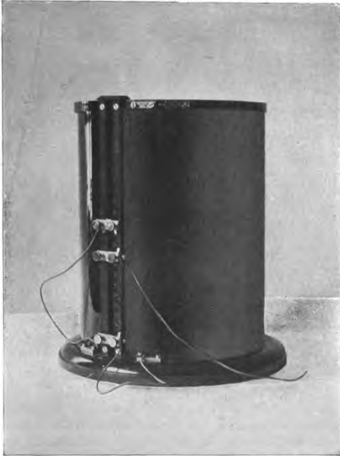
FIG. 65.—Receiving Transformer for Close Coupling.
