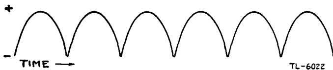
Figure 57. Output of a full-wave rectifier.
