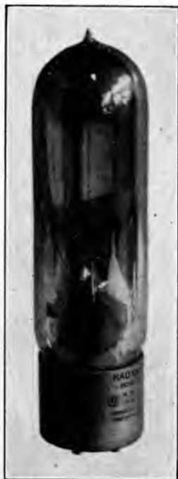
Fig. 74. — Illustrating Radiotron; UV-203; a 50-watt power tube.
