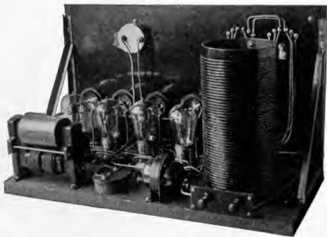
Fig. 106.—Complete low-power radio telephone and c.w. transmitter.
