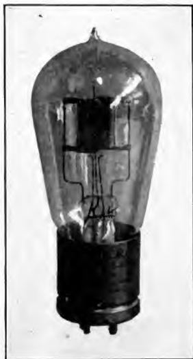
Fig. 75.—Illustrating 5-watt Radiotron; UV-202.
