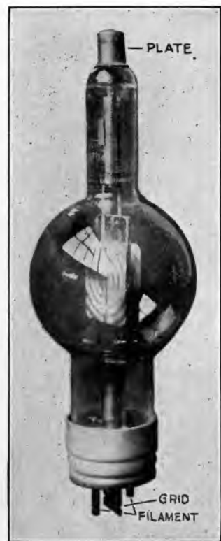
Fig. 73.—Type "P" power tube, prototype of the 250-watt Radiotron; UV-204.
