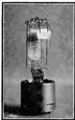
Fig. 29.—View of audion with plane electrodes in which the glass container and part of the electrodes have been removed to show the relation between grid, plate and filament.
