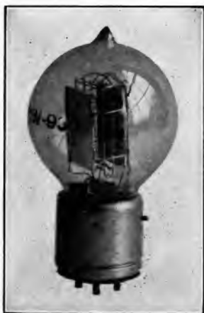
Fig. 76.—Western Electric 5-watt type "E" tube (CW-931 or V.T.-2).
