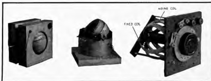
Fig. 8.—Types of variable inductors for radio receiving circuits.
