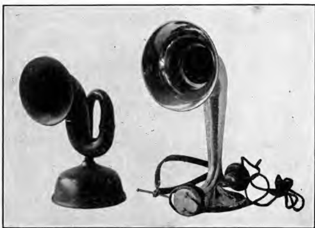
Fig. 152.—Illustrating two commercial sound distributing devices for use with radio telephone-receivers.
