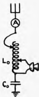
Fig. 83.—Showing connection of microphone to antenna coil for modulating output current in radio telephony (absorption method).
