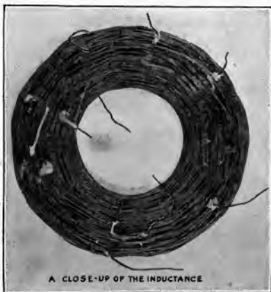
Fig. 126.—Illustrating "spider-web" coil of the Reinartz c.w. receiver.
