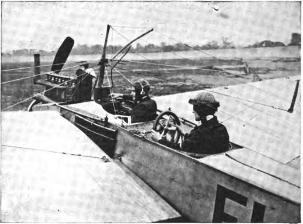
Fig. 325A—Scout Airplane Equipped With Wireless Apparatus.
