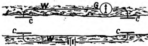
FIG. 3. TELEGRAPHING THROUGH WATER.
