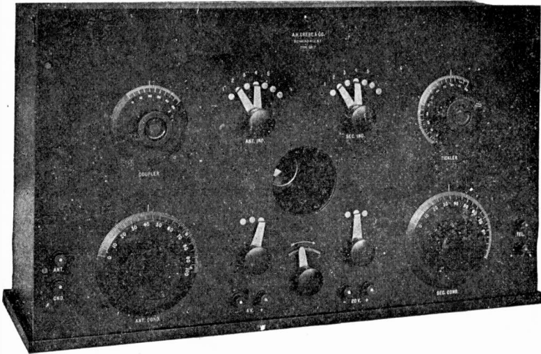
FIG. 207a. Grebe type CR7 long wave receiving set. Range 500 to 20,000 meters.
