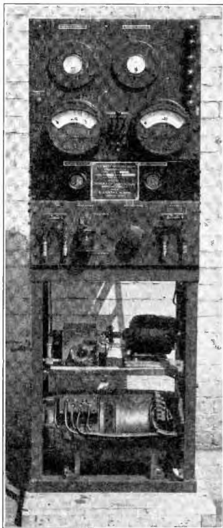
FIG. 257. U. S. Bureau of Lighthouse 100-Watt Radio Beacon Transmitter with Automatic Signalling Device.
