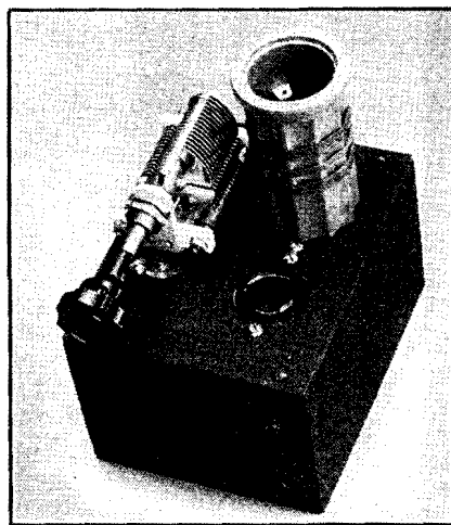
Fig. 1046 — Compact plug-in type antenna tuner for low-power transmitters. The tuning condenser is insulated from the chassis by means of a pair of National FWB terminal strips. The front socket is for parallel tuning, the rear one for series tuning. The clearance hole at the rear of the condenser is for the connection to the condenser stator. The rotor connection is taken off underneath.
