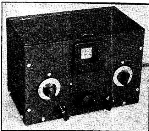
Fig. 819 — Front view of the converter. The hand-spread knob is at the center with the band-set and detector tuning condensers to the right and left, respectively. The antenna and on-off switches are to the left and right at the bottom of the panel.
