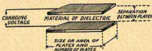
FIG. 4.—The Four Factors Affecting a Condenser's Charge.
