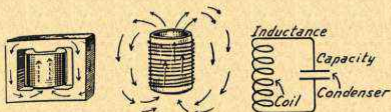
An Oscillatory Circuit.
