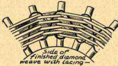
Fig. 3.—Lacing the Finished Diamond Weave Spiderweb Coil.
