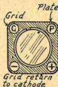
Fig. 3.—Socket Connections for Heater Tube.
