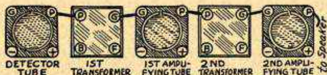
FIG. 4.—Audio Amplifier with Output at Right.
