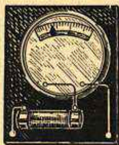
FIG. 5.—Milliammeter Used as Voltmeter.
