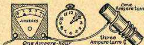
Ampere-Hour and Ampere-Turn.
