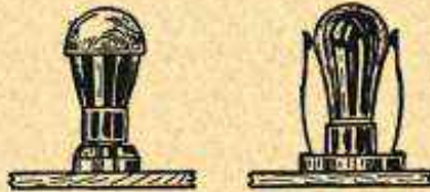
Noise Prevention with Devices for Deadening Vibration in Tubes.
