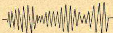
FIG. 3.—Carrier Modulated with Sound Frequency.
