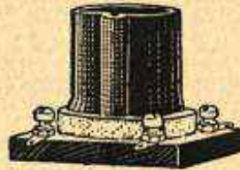
FIG. 6.—Socket Mounted on Sponge Rubber.
