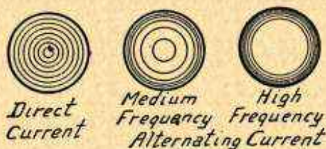
Skin Effect on Current Distribution in Wires.
