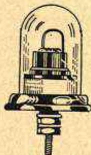
FIG. 4.—Crystal Detector with Fixed Cat Whisker.
