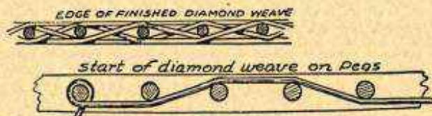
FIG. 2.—Method of Winding Diamond Weave Spiderweb Coil.
