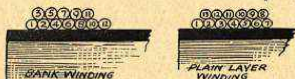
FIG. 1.—Bank Winding of Two-Layer Coil.
