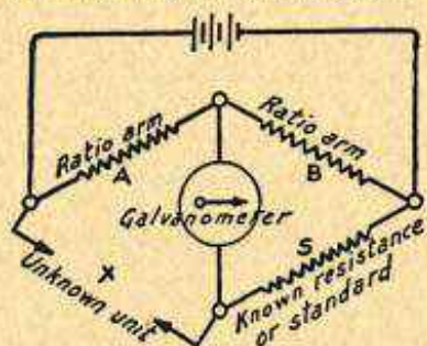
FIG. 3.—Functions of the Arms in a Bridge.
