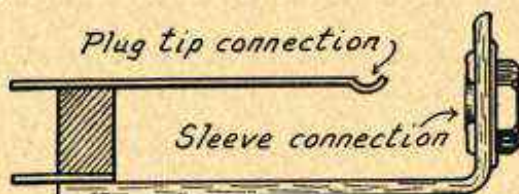
FIG. 3.—Mounting Bracket Used as Sleeve Connection for Jack.
