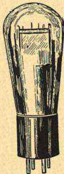
FIG. 4.—Large Type of Power Amplifier Tube.
