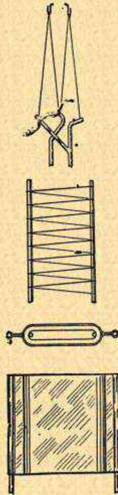
FIG. 5.—Design of a Half-Ampere Power Tube.
