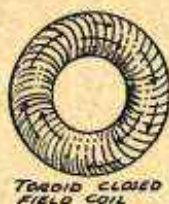
FIG. 1.—Toroid Type of Coil.
