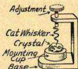
FIG. 3.—One Form of Crystal Detector.
