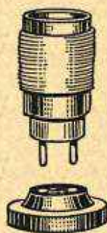
FIG. 2.—Plug Mounting for Coil.
