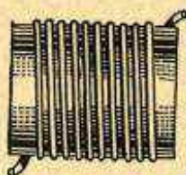
Space Winding on Single Layer Coil.
