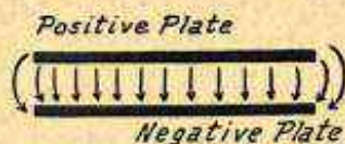
FIG. 1.—Electrostatic Field between Condenser Plates.
