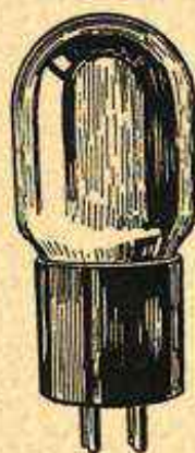
FIG. 3.—Amplifier Tube with Cylindrical Bulb.
