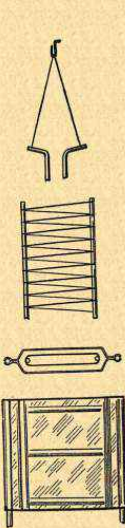
FIG. 4.—Design of a Semi-Power Tube.
