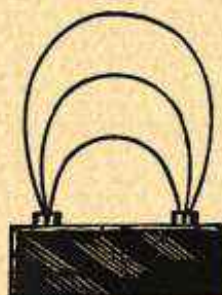
FIG. 1.—Circuits with Resistances in Parallel on Battery.
