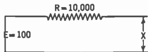
FIG. 28. —A low resistance voltmeter placed at X will not read the open circuit voltage.
