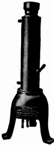
FIG. 38.—The Langmuir Mercury Vapour Pump.
