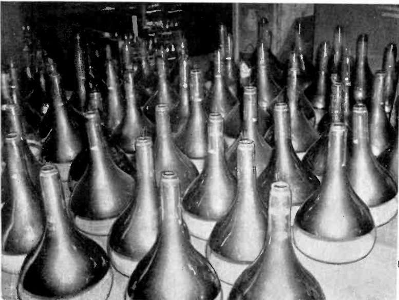
With the advent of commercial television, these 14-inch Du Mont teletrons became a production item rather than a laboratory masterpiece. Dozens of the 14-inch and 20-inch teletrons are produced each working day in equipping as many Du Mont television receivers.
