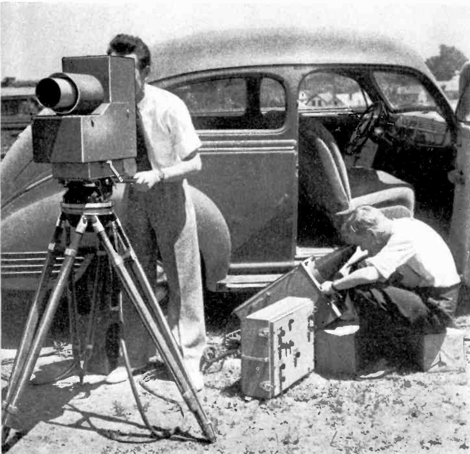
Recognizing the wide range of television program circumstances, the Du Mont organization decided on the unit plan of assembling required "chains". In other words, a choice of standard, portable, self-contained units is available. These are connected together to form a "chain" to meet the program needs, either for outside pickup or for studio use. This is some of the earlier equipment, prior to the electronic view finder feature.
