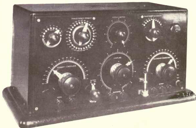
A special panel receiving set was also designed for use in ship work. The photograph shows the type 106 receiving tuner of the American Marconi Company which is complete in every detail. It has a range of wave length from 200 to 3,500 meters and is particularly suitable for ship traffic. The cabinet contains the component parts of an inductively coupled receiving transformer with all accessory apparatus necessary for tuning and adjusting. The tuner also includes a buzzer tester for preadjusting the crystal to its most sensitive condition.
