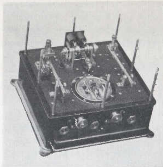
FIG. 517. Marconi Auto-Alarm Selector with Cover Off, showing Relay Ratchet and Pawl Systems and Contact Arms.
