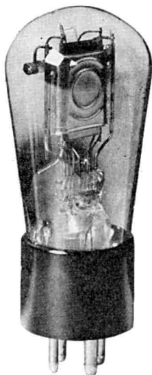
FIG. 39. A three-electrode high-vacuum tube designed to have a minimum of undesired disturbances in the plate current flow; that is, a "low-noise" tube.
