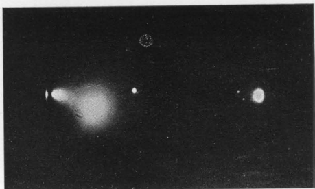
FIG. 21.—NON-LUMINOUS ARC IN PURE MERCURY VAPOUR IN A LARGE VESSEL.
