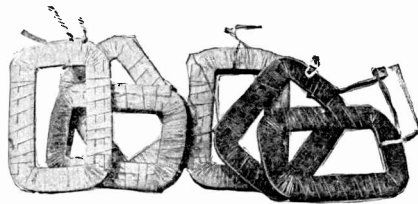
Fig. 266. Sample Coils for Fort Wayne Transformer
