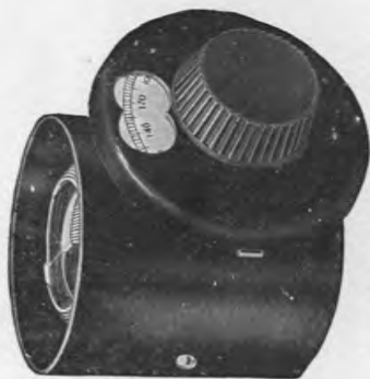
Complete Variometer enclosed in ebonite protecting tube.
