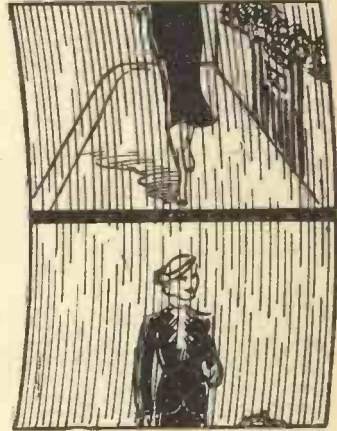
Fig. 45—A movement of the pole pieces of the synchroniser suffices to cure the fault shown above, which only occurs when synchronising gear is used
