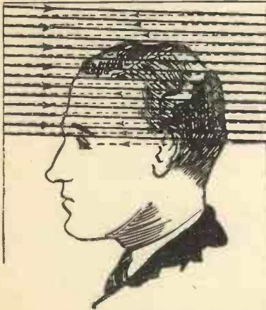
Fig. 18—Showing how the scanning spot traverses a picture or a "subject," being bright where the picture needs to be bright and dark where the picture needs to be dark, and so building up the picture
