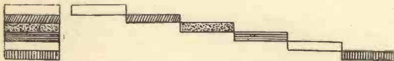
Fig. 85—This diagram shows how the picture is split up into a straight line before scanning in the Scophony principle of television, which calls for scanning in one direction only
