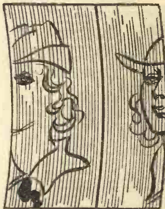
Fig. 42—The condition shown above results from the scanning being out of phase, although the motor is running at the correct speed
