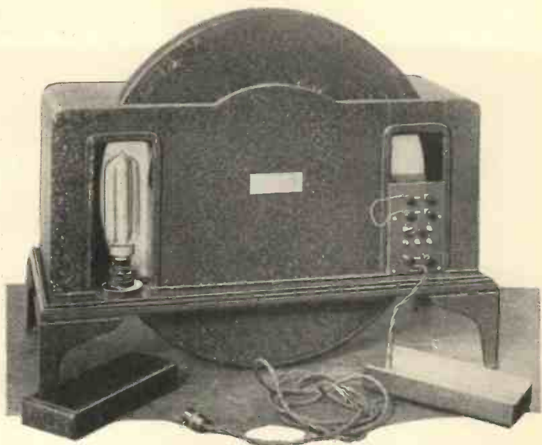
A BACK VIEW OF THE BAIRD TELEVISOR FOR LOW DEFINITION TELEVISION. ON THE LEFT CAN BE SEEN THE NEON LAMP IN FRONT OF WHICH RUN THE HOLES IN THE ROTATING SCANNING DISC
