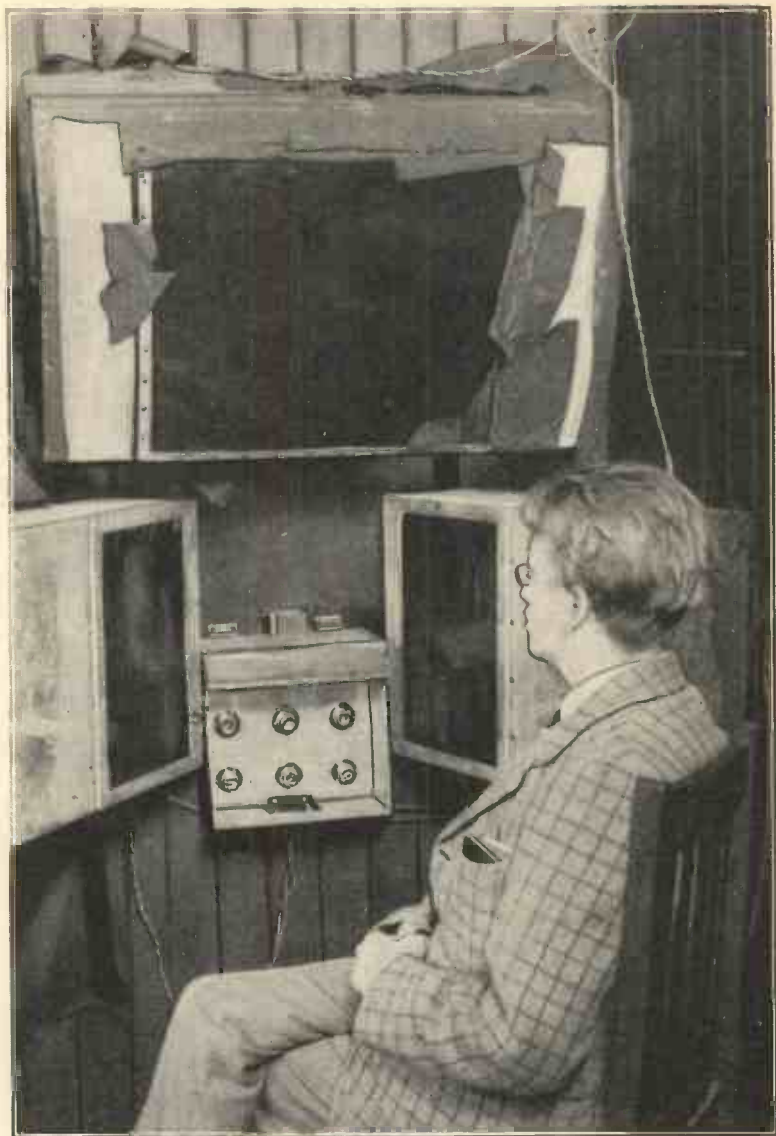
TELEVISION WITHOUT THE AID OF VISIBLE LIGHTING. BAIRD AND AN APPARATUS EMPLOYING INFRA-RED RAYS WHICH HE DEMONSTRATED MANY YEARS AGO
