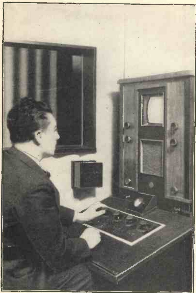
THE CONTROL PANEL OF THE TELEVISION EQUIPMENT AT BERLIN. TRANSMISSION IS ON ULTRA-SHORT WAVES FROM THE WITZLEBEN STATION
