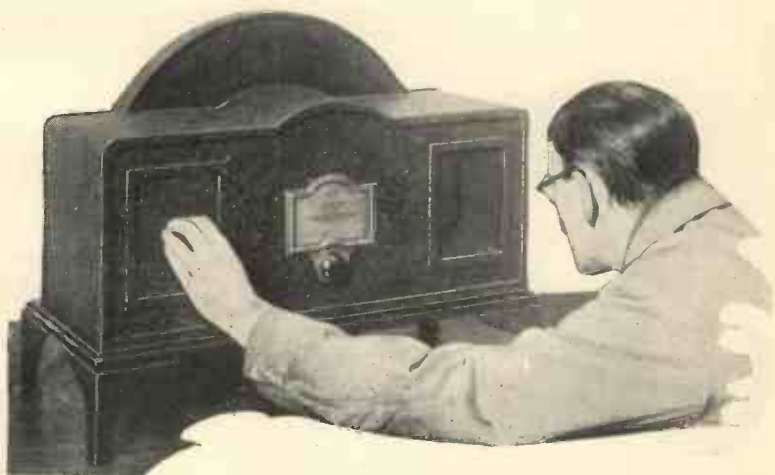
THE BAIRD TELEVISOR WHICH WAS SOLD FOR THE RECEPTION OF THE LOW DEFINITION PROGRAMMES. THE OPERATOR IS SEEN ADJUSTING THE FRAMING OF THE PICTURE
