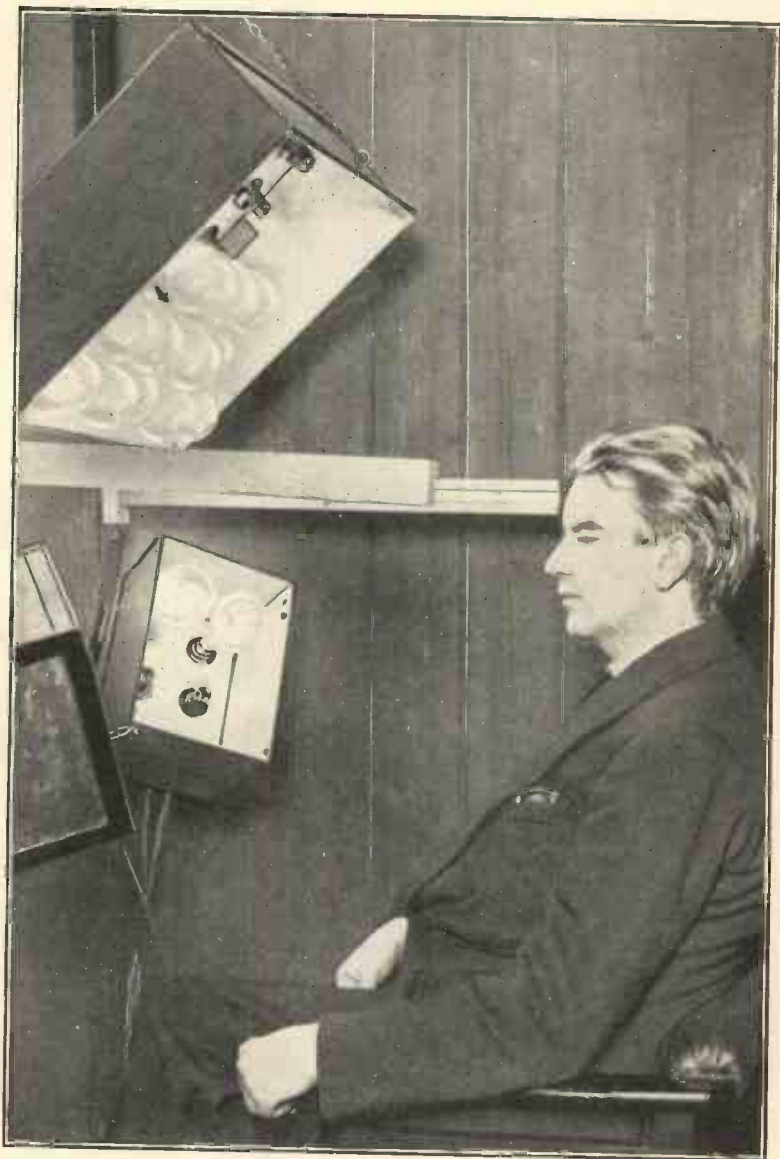
AN INDICATION OF THE INTENSELY BRIGHT FLOOD-LIGHTING NECESSARY IN THE EARLIER DAYS OF TELEVISION IS PROVIDED BY THIS PHOTO OF BAIRD HIMSELF BEING TELEVISED BY ONE OF HIS FIRST TRANSMITTERS
