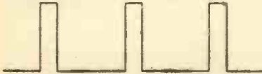
Fig. 131—The synchronising impulses are sent out at greater modulation than the picture frequencies, and are fairly flat in form. In practice many systems keep the minimum modulation strength for the picture impulses up to, say, 30 per cent of the carrier, and then send the synchronising impulses as complete drops to zero instead of a build-up of modulation. In other words, the diagram shown in Fig. 132 is turned upside down, the dotted line denoting the 30 per cent line. The result on the synchronising valve is, of course, the same—a powerful A.C. impulse
