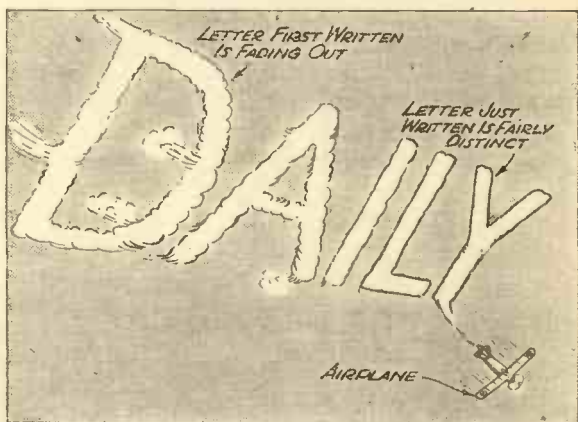
Fig. 11—The pilot has written the word "Daily," but, owing to the effect of the wind, the letters which were first written are fading out, whilst those which he has just done are much clearer. The same kind of thing happens with the light-spot which builds up the received picture in television. To avoid it, the light-spot must travel very quickly
