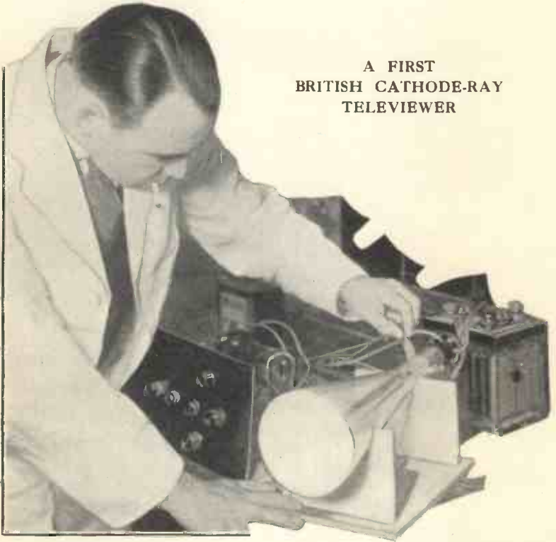
A "POPULAR WIRELESS" TECHNICIAN DEMONSTRATING THE FIRST SUCCESSFUL BRITISH CATHODE-RAY RECEIVER. THIS TUBE WAS OPERATED ENTIRELY BY BATTERIES
