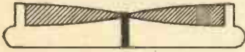
Fig. 203—Stereoscopic photos are viewed through two separate eye-pieces, each consisting of a wedge-shaped lens
