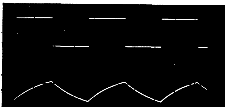
Fig. 5-2. Effect of integration. (A) On a sine-wave. (B) On a triangular wave. (C) On a square wave.
