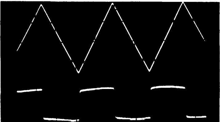
Fig. 5-4. Effect of differentiator. (A) On a sine wave. (B) On a square wave. (C) On a triangular wave.
