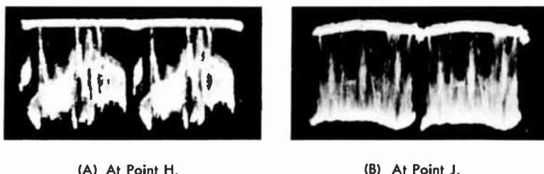
Fig. 9-5. Waveforms Observed in the Circuit of Fig. 9-2 When R4 of Fig. 9-1 Is Open.
