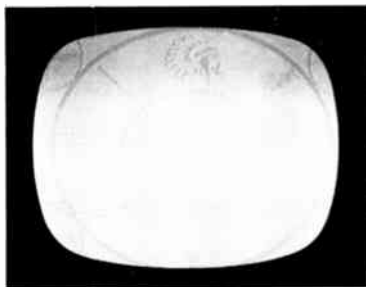
(B) Weak Picture Produced by Excess of Bias to All Controlled Stages.
