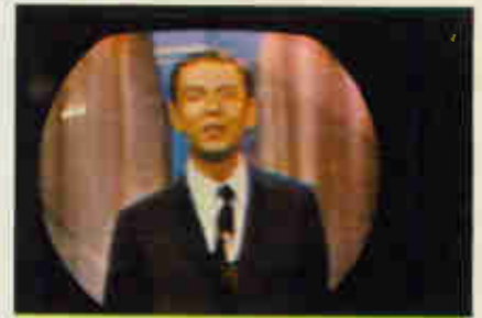
Fig. 5. Lead too close to antenna mast.
