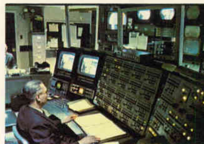
Monitors show input and "round robin" signals. Switcher times various events.
