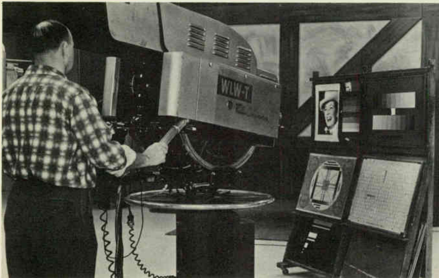
Fig. 1. Studio color camera being adjusted with aid of scale charts on stand.
