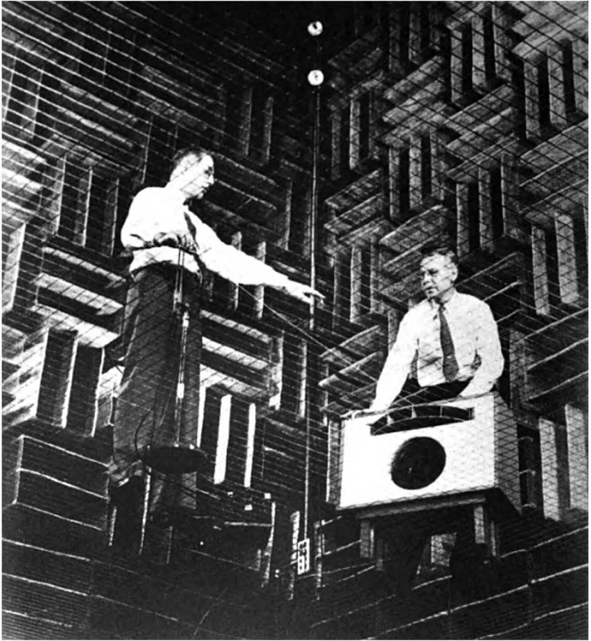
Fig. 11-13. Measurement of performance characteristics of a loudspeaker in an acoustically "dead" room which has been treated to minimize all reverberation to the greatest possible degree.
