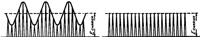
Figs. 19, left, and 20. The average value of the carrier voltage is the same, whether the signal is modulated (Fig. 19) or unmodulated (Fig. 20).
