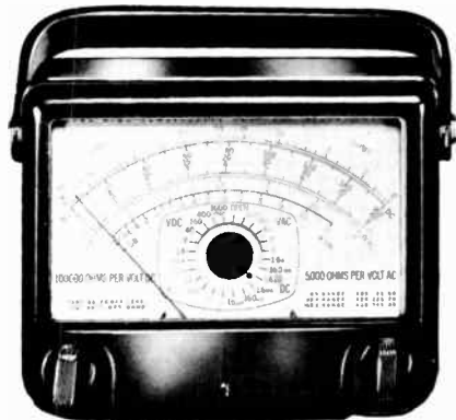
Fig. 1-7. High sensitivity VOM—measures 16 \mu a full scale.
