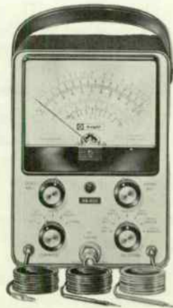
Fig. 1-2. Knight-Kit Model KG-620 VTVM.
