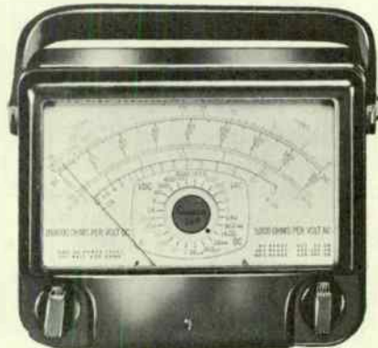
Fig. 1-7. High sensitivity VOM—measures 16 \mu a full scale.
