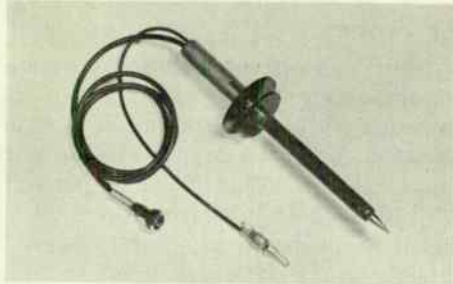
Fig. 2-12. High voltage probe containing multiplier.
