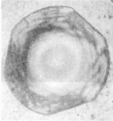
b. Top view of indium dot showing triangular shape.
