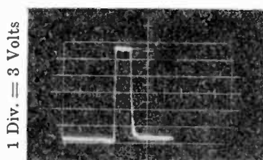
1 Div. = 3 Volts 1 Div. = 5 \mu Sec (a) Horizontal rate.
