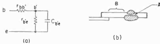
Fig. 1—(a) Equivalent input circuit of the transistor and (b) Transistor cross section showing the physical location of the parts of r_{bb'} on a TA-153 audio-transistor.
