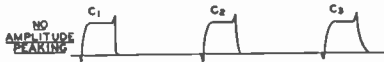
Fig. 8—Effects produced on a square wave by the introduction of various values of capacity in the phase shifting sections.
