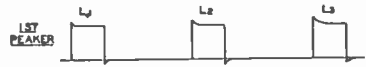
Fig. 6—Effect produced on a square wave with the peaker potentiometer open for various values of inductance (first peaker).
