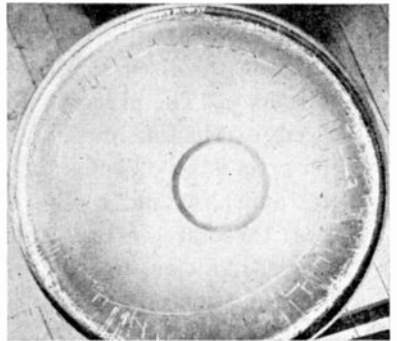
Fig. 4—Pressure test failure.
