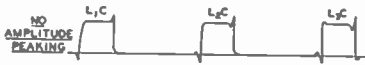
Fig. 10—Effects produced on a square wave by the introduction of various values of inductance in series with additional capacity in the phase shifting sections.
