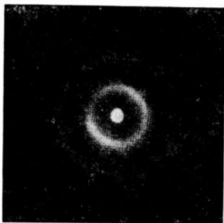
Fig. 3—Appearance of stationary spot on kinescope screen illustrating series of concentric circles of illumination occasioned by halation.
