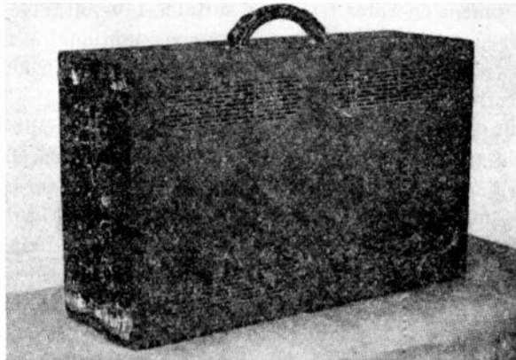
Fig. 4—Synchronizing-generator shaping unit with covers in place.
