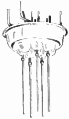
Moulded glass stem assembly showing individual lead seals.
