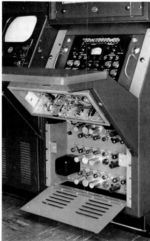
FIG. 35. The modulation shading amplifier is mounted beneath the desk section of the processing amplifier.
