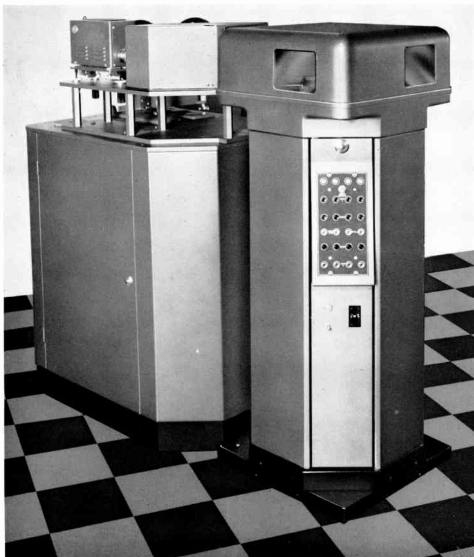
FIG. 10. TP-15 Multiplexer main pedestal (right) contains mirror assembly and control panel; auxiliary pedestal provides mounting for 1-V camera and slide projector.
