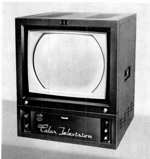
FIG. 1. TM-21 Color Control Monitor. Only operating controls normally exposed are brightness, contrast and on-off switch.
