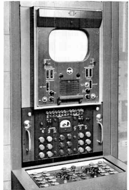
FIG. 4. Alternative mounting of master monitor, processing amplifier and camera control in 84-inch rack combined with accessory desk.
