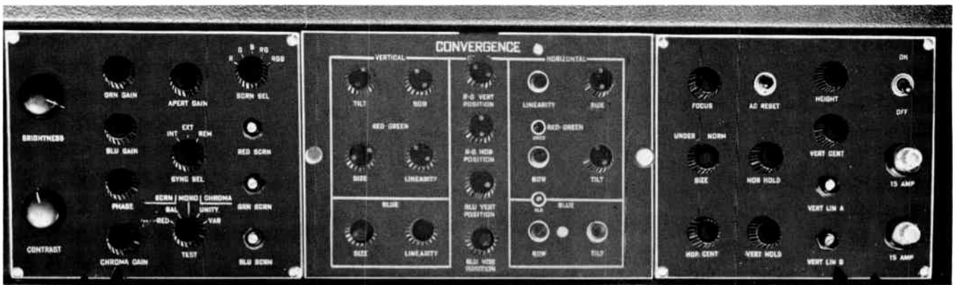
FIG. 18. Close-up view of control section. Located left to right are deflection, convergence and decoder control panels.
