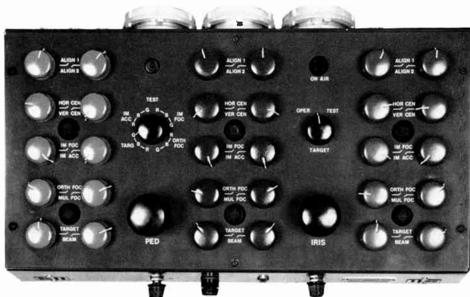
FIG. 9. View of camera control panel showing setup and operating controls.
