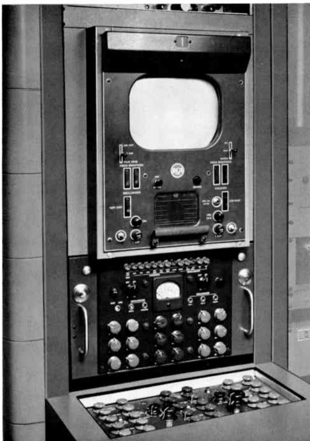
FIG. 5. Alternative method of mounting processing amplifier and master monitor in a standard cabinet rack. Camera control is shown in desk below amplifier.
