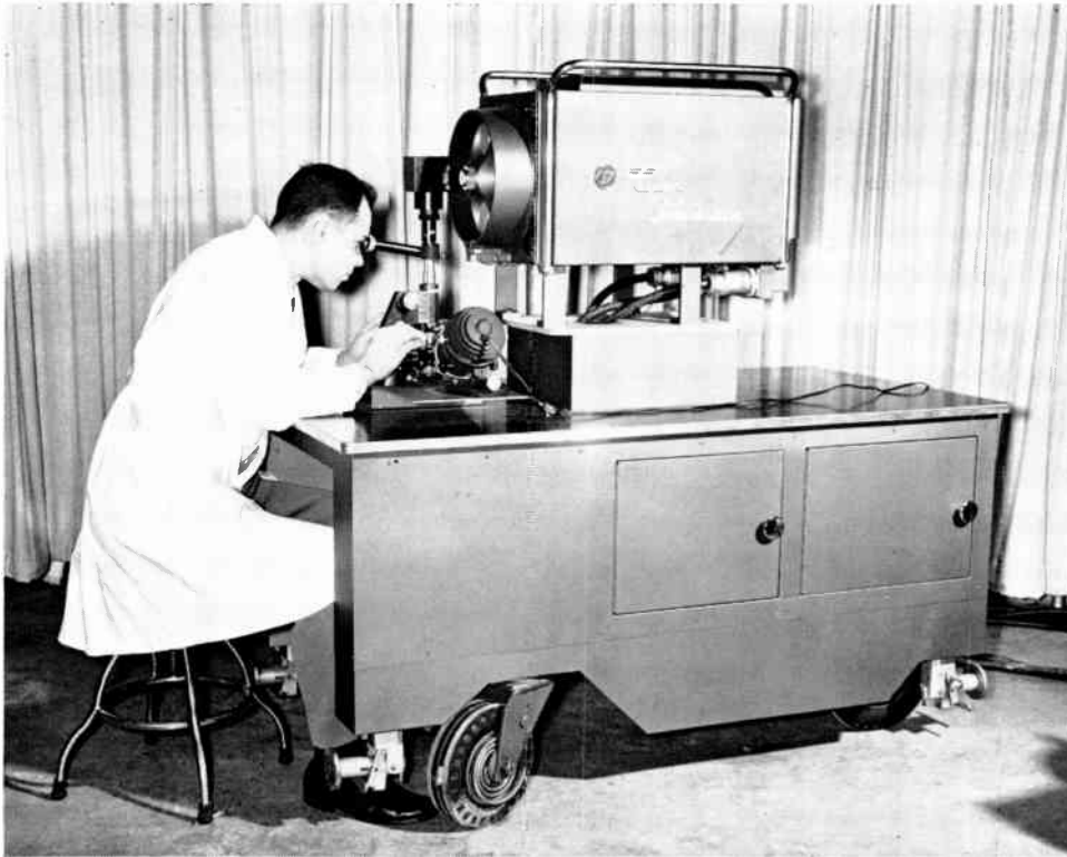
FIG. 23. The three-vidicon color camera used in conjunction with optical microscope for group demonstrations.
