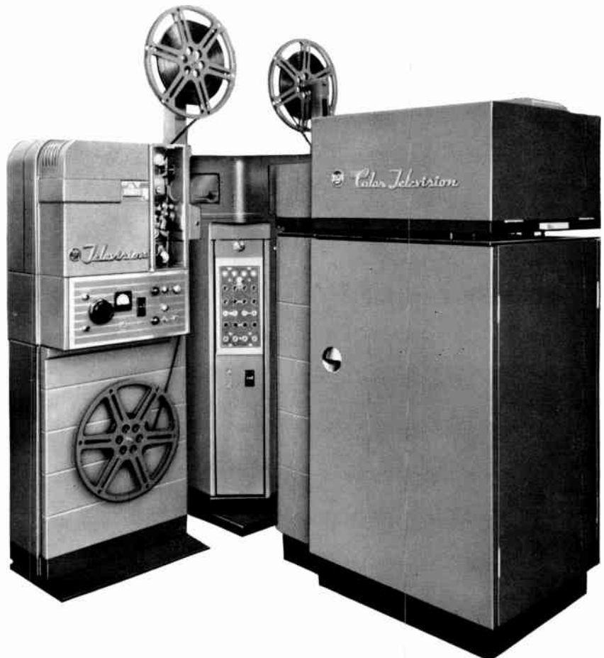
FIG. 3. Projection room equipment consists of film camera, two film projectors, multiplexer (center) and slide projector located on opposite side of multiplexer.
