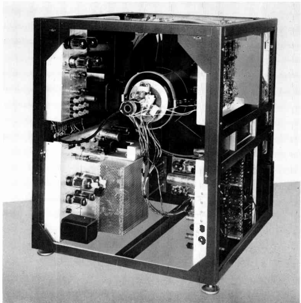
FIG. 3. Rear-quarter view of TM-21 with side and top covers removed, showing how the chassis are mounted within the main frame.
