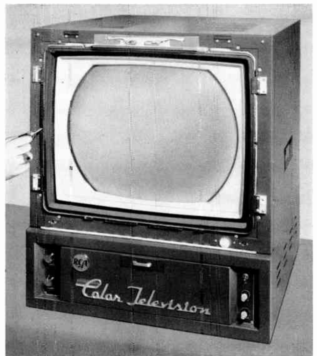
FIG. 5. Decorative bezel surrounding the picture area is removed for access to the equalizing magnets and the safety glass.
