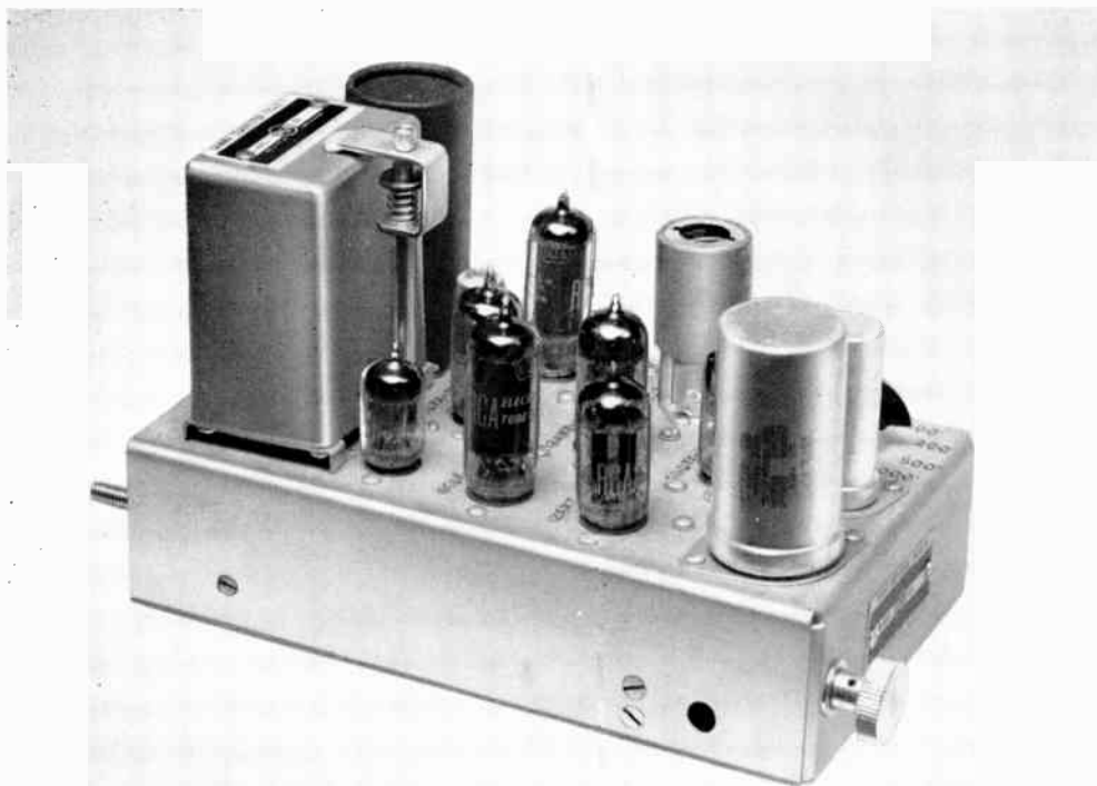
FIG. 36. The video amplifier in the processing amplifier contains a plug-in gamma compensation unit (left side of chassis) with a 0.7 gradient correction.
