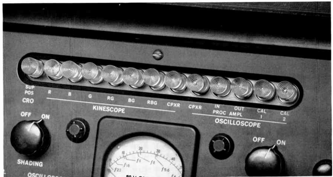
FIG. 12. Closeup view of processing amplifier showing pushbutton selection switches.
