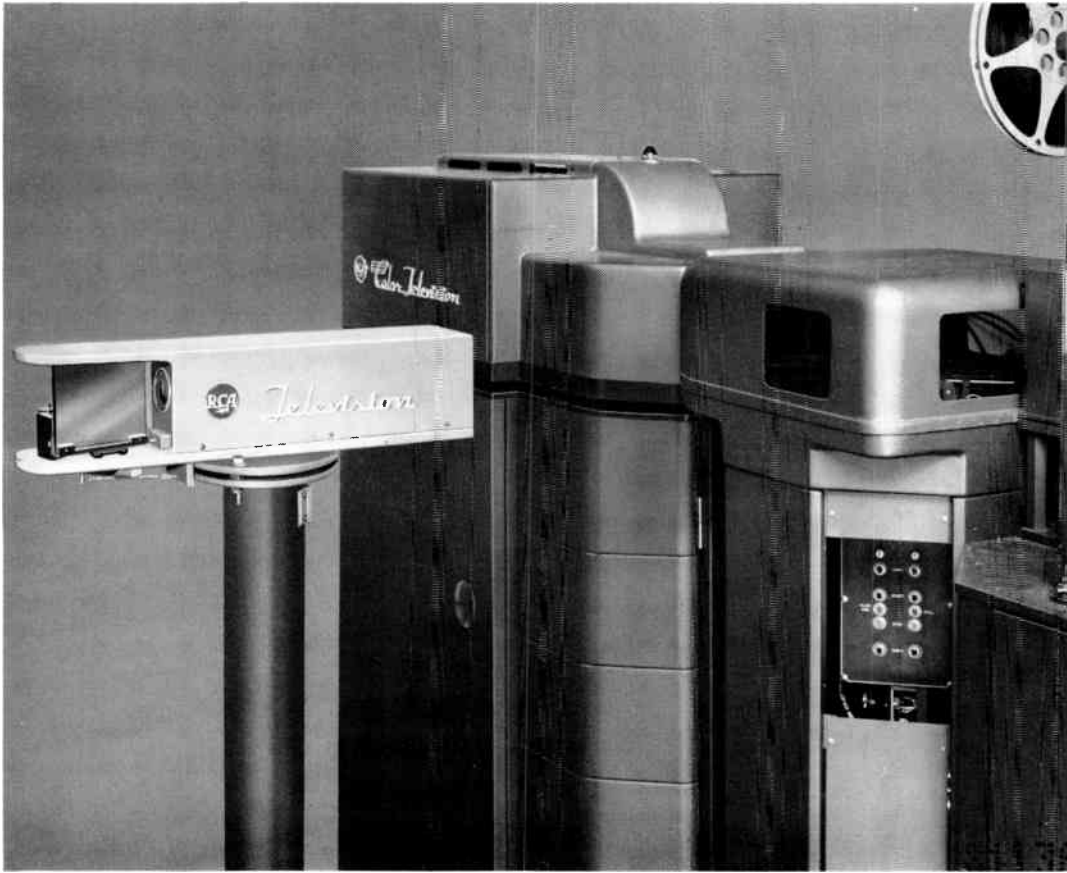
FIG. 26. Opaque Pickup Assembly mounted facing TP-15 Multiplexer.
