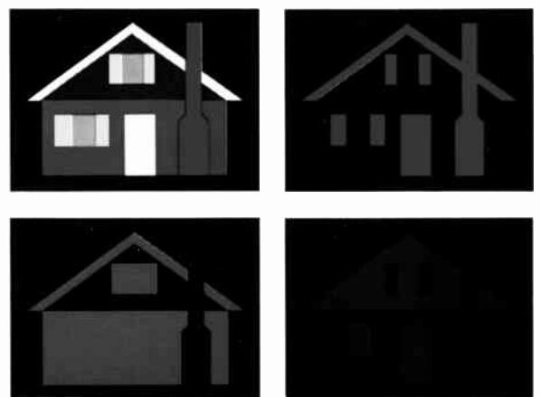
FIG. 10. Illustrating how a typical color image (upper left corner) can be separated by optical means into red, green and blue image counterparts.
