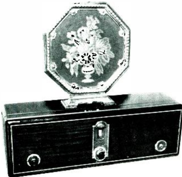
Radiola 17 , the first ac radio. The receiver contained six tubes plus rectifiers and operated on a tuned radio frequency principle.
