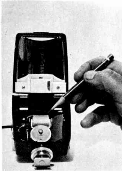
The bulb is in top, generator wheel in the lower half of Kodak Generator Flashholder's hinged case. Pencil points to generator's fixed winding; magnet turns below it. Hook-up is diagrammed, right.
