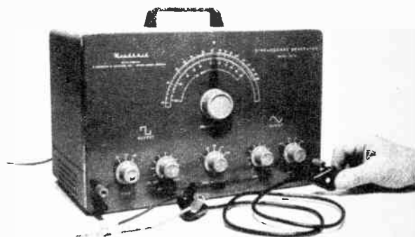
Front panel of the completed Heath AG-10. Upper central knob is tuning for different frequencies. Other knobs adjust strength of output signals.
