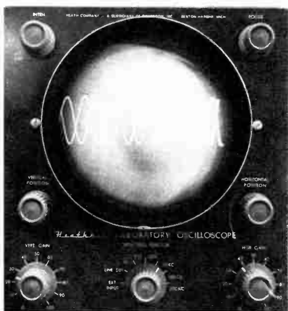
Compound and complex signals can be "seen" because electron spot moves extremely rapidly and the trace it makes on the fluorescent screen of C. R. tube lingers for a fraction of a second.
