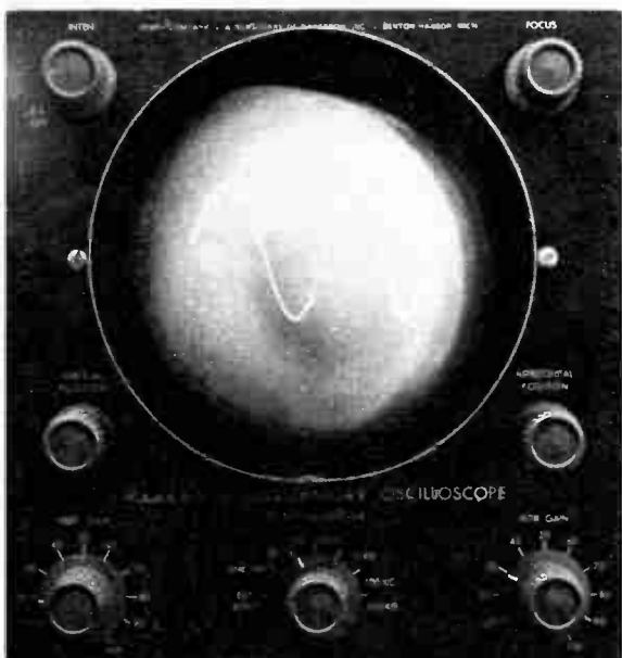
Number of AC cycles produced on C. R. tube is ratio of input signal frequency to sweep frequency. Here the input is 60 cps but sweep has been reduced to 30, for two "sine wave" shapes.
