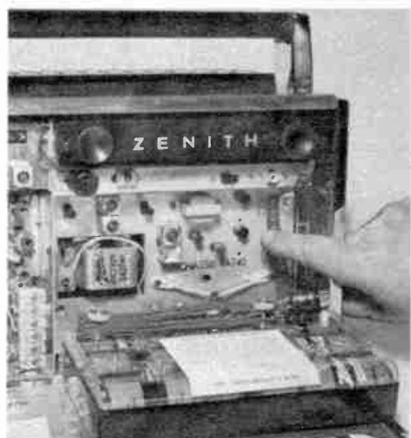
Rear view, with cover lowered. Finger indicates one of nine tiny transistors. Note flashlight batteries in transparent case within the cover.
