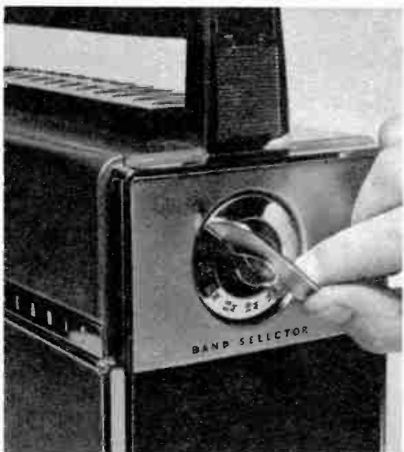
Band selector switch is located in right end of the case. Key-type knob folds flat when not needed to prevent it from snagging clothing, etc.
