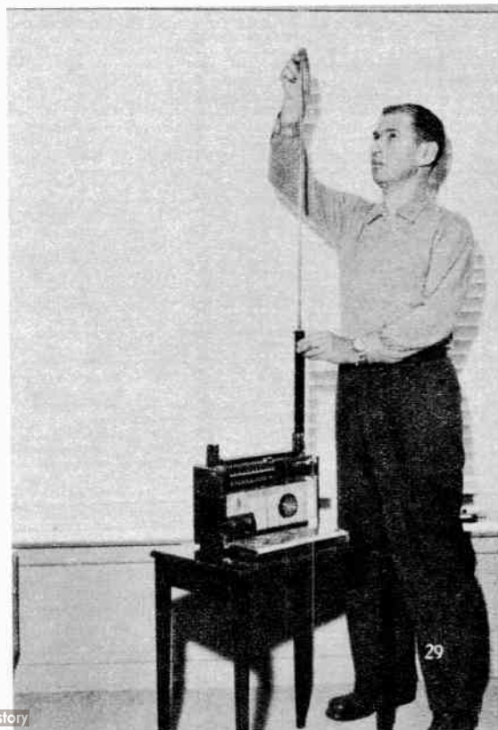
Telescoping rod antenna, ingeniously concealed in handle of case, is for short-wave reception. Spring lock keeps it secure in the upright position.
