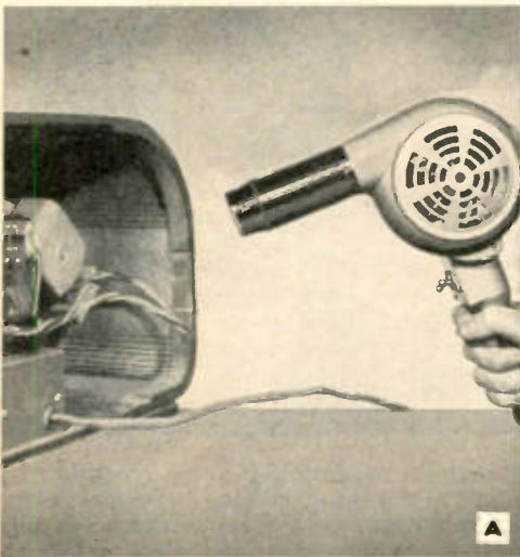
Photo A —Dust collects inside every radio receiver as there is no way to keep it out and provide the necessary ventilation. A small power blower may be used to remove dust from the top of the chassis as illustrated. In this case a hair drier is used; it provides a blast of air to remove the dust and heat to dry out moisture.
