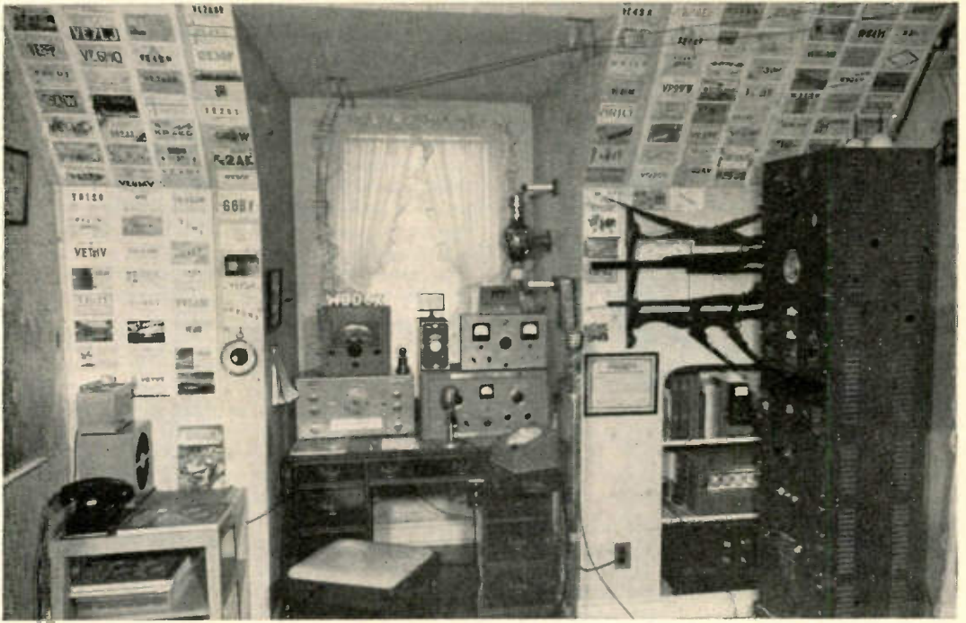
Above, operating position at W9DCX; the direction indicator unit for monitoring the position of the beam antenna is on the desk slide arm. A 400-watt, 10-meter phone and c.w. transmitter is located at the right. Below, left, rotary beam antenna operated by remote control. Lower right, 1-kw. 20-meter phone transmitter
