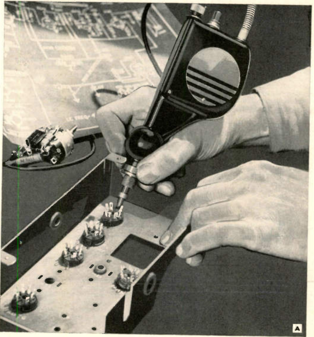
MARKING CHASSIS BASE TO IDENTIFY TUBE SOCKETS
