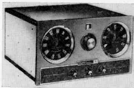
Stereo tuner model 3304 made by Electro-Voice can replace separate AM and FM tuners in systems for receiving broadcast AM-FM stereo.
