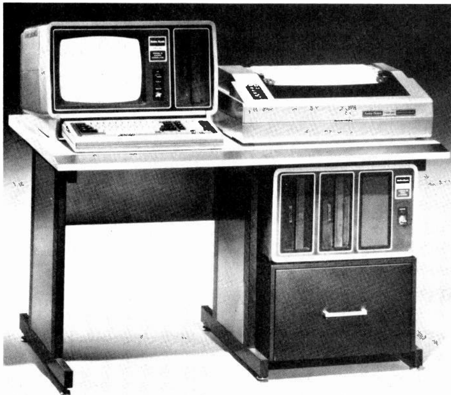
Radio Shack TRS-80 Model II microcomputer with Line Printer III, external 8-in. floppy-disk drive system, and system desk.
