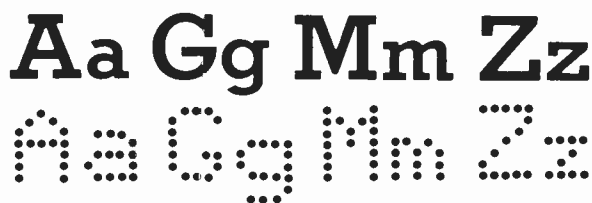
Examples of formed-character and dot-matrix printing. Note difference in legibility.
