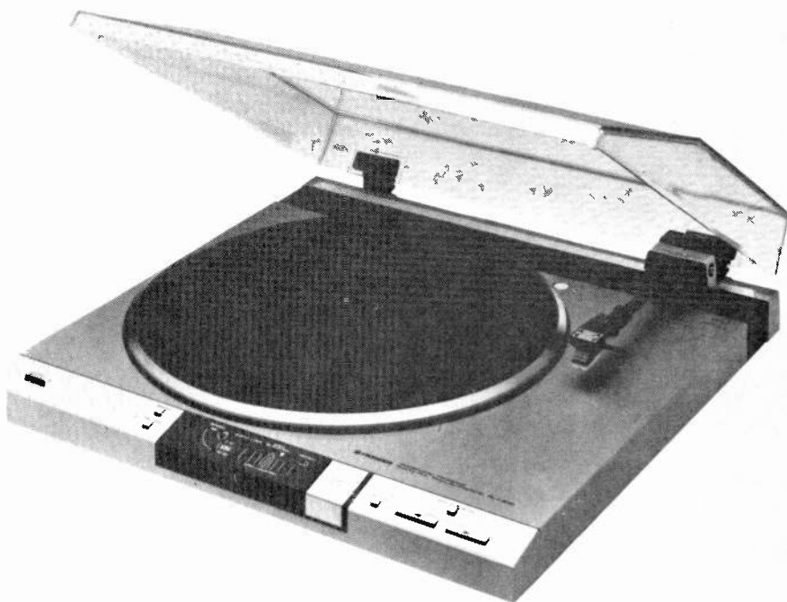
Pioneer PL-L800 linear-tracking turntable with up-front controls.
