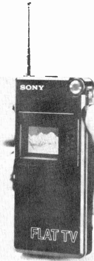
Sony FD-200 pocket TV set uses a liquid-crystal picture "tube".
