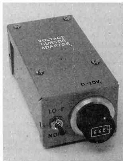
THE CURSOR ADAPTER superimposes horizontal cursor lines on the top and bottom of a waveform.
