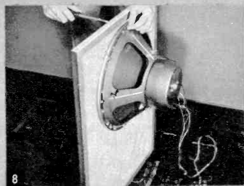
6 LOUDSPEAKER is next mounted on front panel. GRILLE CLOTH installation completes assembly.
