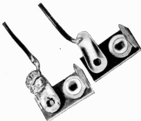
COLD SOLDER joint (left) has obviously poor appearance as compared with correct joint (right).
