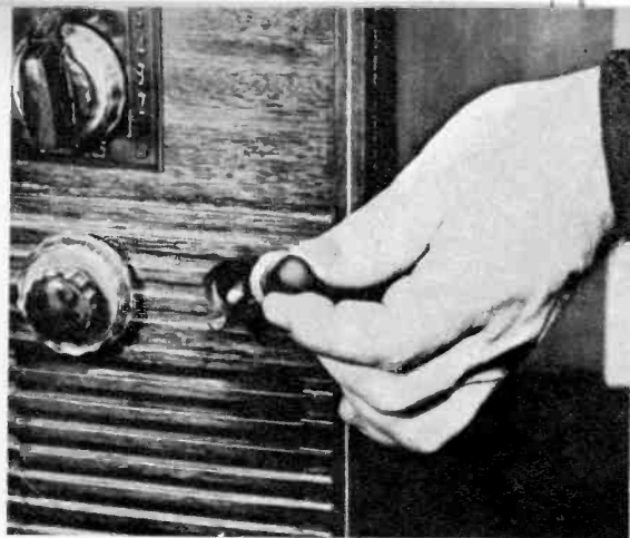
REMOVE KNOB , tilt set slightly backward, let fluid run down the shaft. Work in by rotating shaft.
