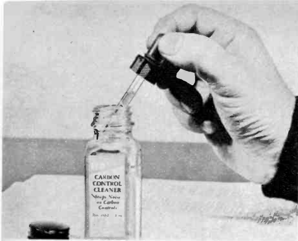
CLEANER for carbon-type variable controls is a special solvent. Apply it with an eye dropper.
