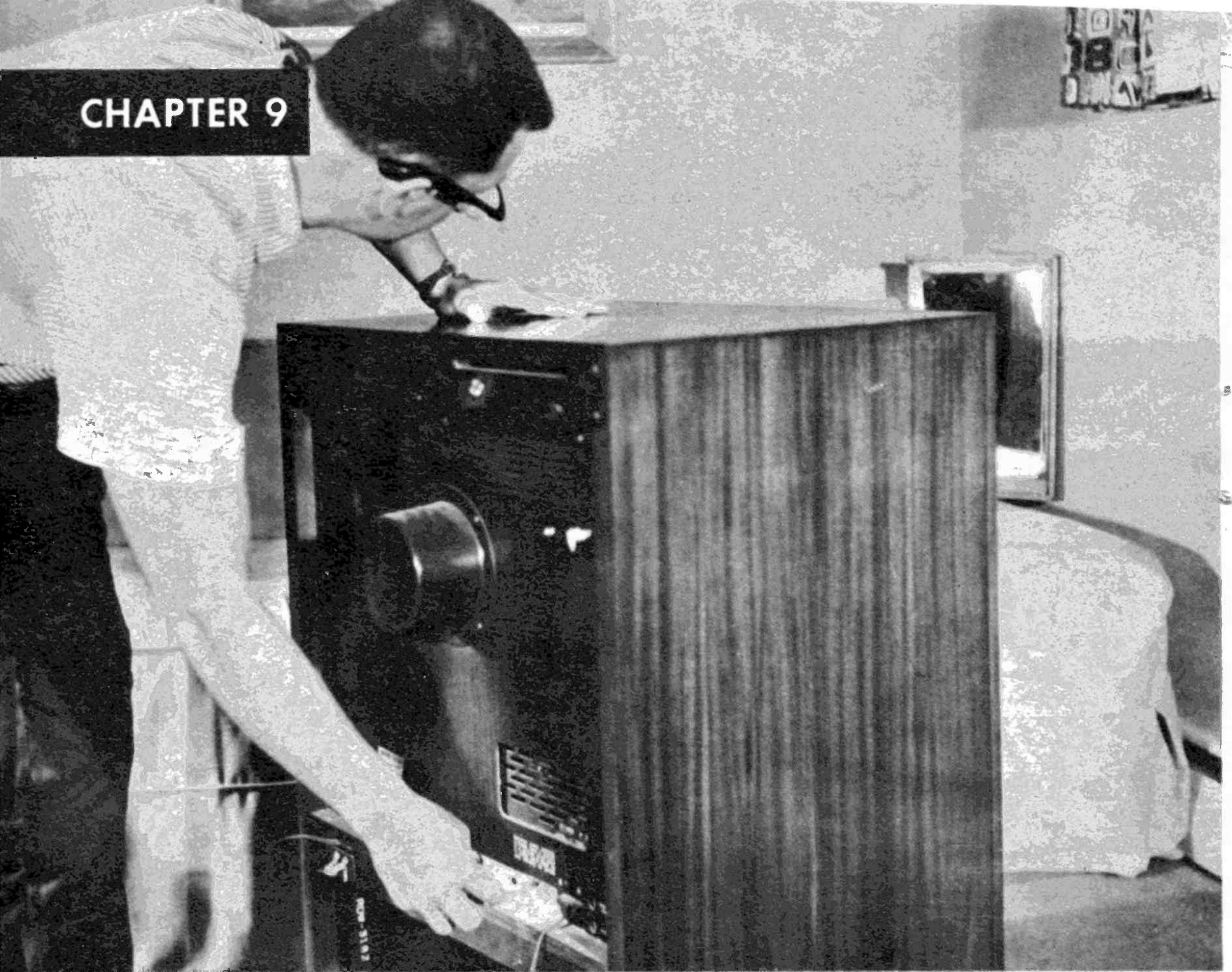
Adjustment of the AGC control on the TV set turns the picture signal from washed out to overly black.
