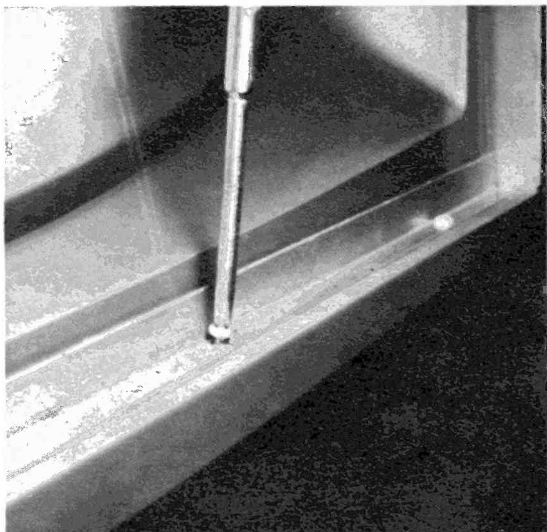
Many TV sets have built-in provisions to remove the safety glass for cleaning. Look for screws.
